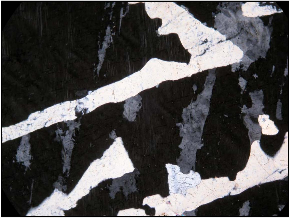
Figure 44c. A photomicrograph of a thin section of an igneous intrusive rock (6.i), showing the graphic quartz intergrowths within perthitic microcline. Long axis of photomicrograph = 4 mm. (SR1299).
