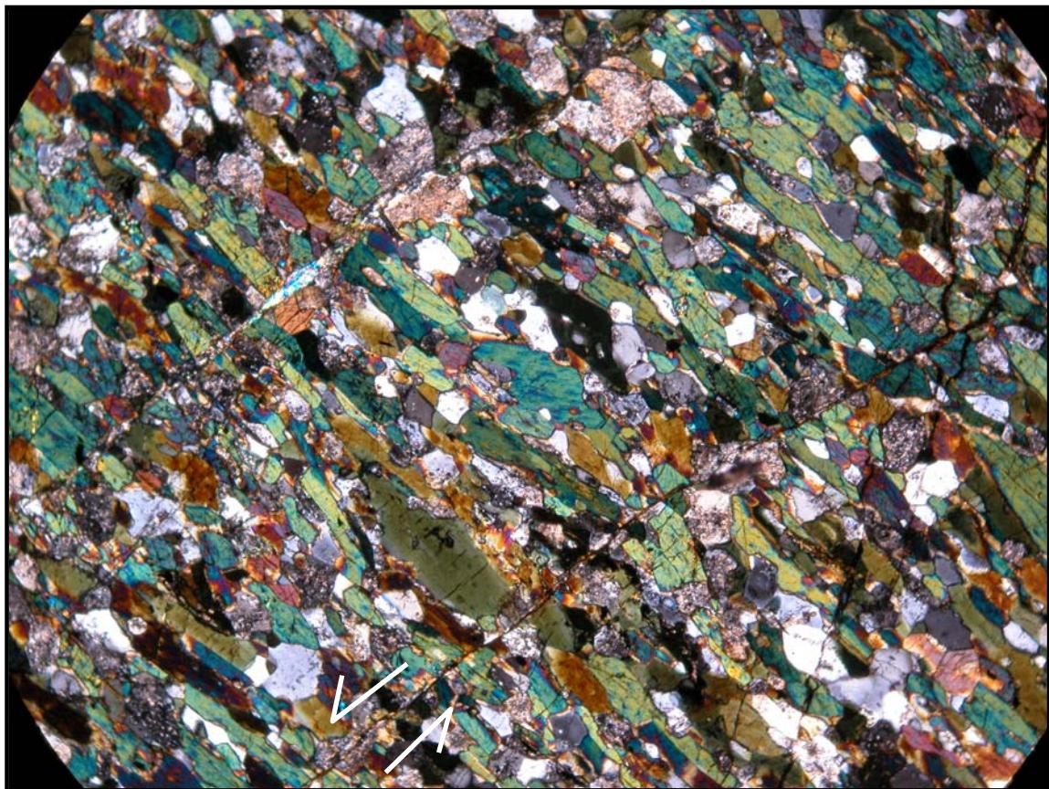
Figure 66. A photomicrograph of a thin section showing extensional feature. Long axis of photomicrograph = 4 mm. (NR2699).
