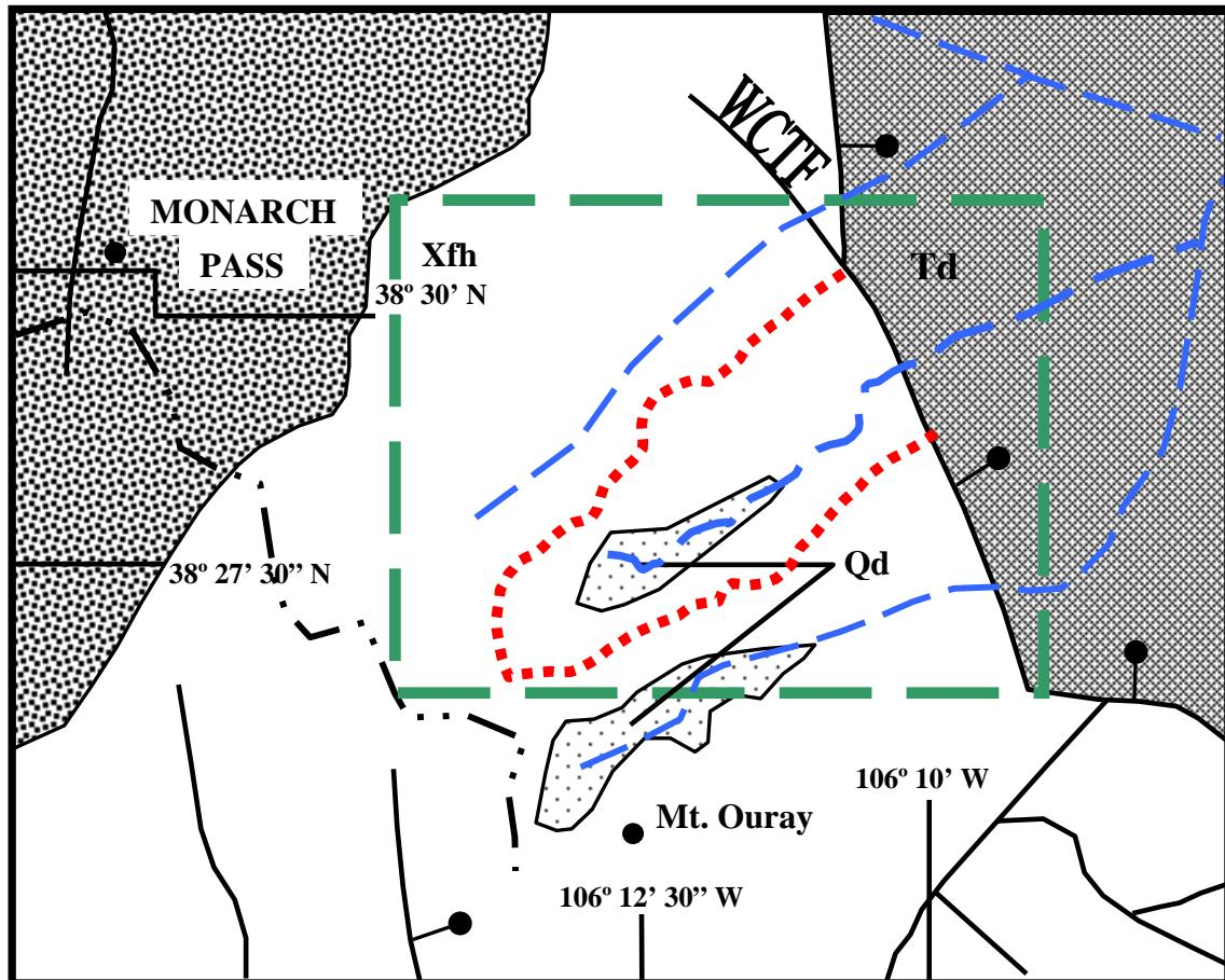
*Figure 45. Simplified geologic map of South-Central Colorado showing Field Area (dashed rectangle), ridgeline traverse (dotted line) and three primary units of Xfh (Precambrian Felsic and Hornblendic Gneisses), Td (Tertiary deposits east of the WCTF) and Qd (Quaternary deposits within the Pass Creek and the Little Cochetopa Creek drainages). Also shown is the Monarch Pass (Proterozoic granite YXg) (modified from Tweto, 1979).*
