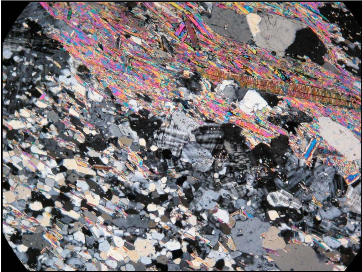
Figure 44g. A photomicrograph of a thin section of the quartz mica schist “whiteschist” ( $3e.Xfh:Xqms$ ). Long axis of photomicrograph = 4 mm. (NR13a99)
