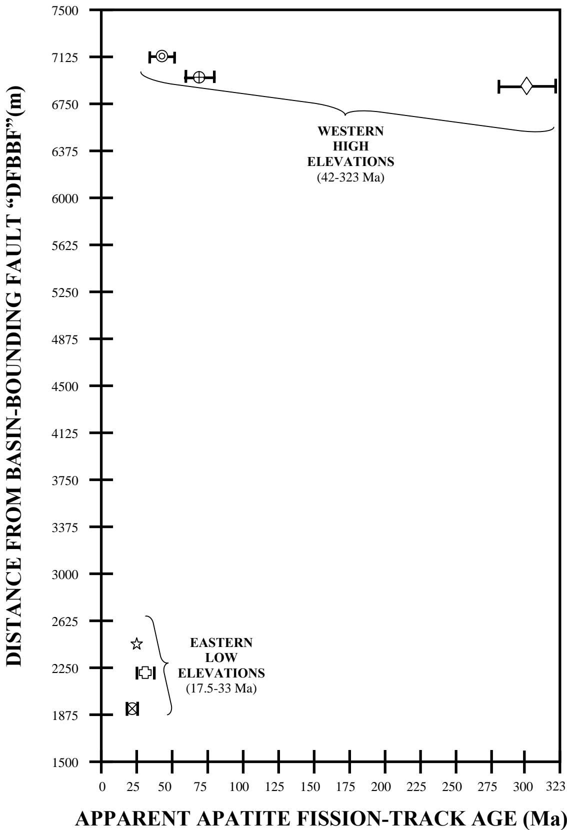
Figure 78. Age (Ma(BP)) versus Distance From Basin-Bounding Fault (“DFBBF”)(m) plot of AFT results.
