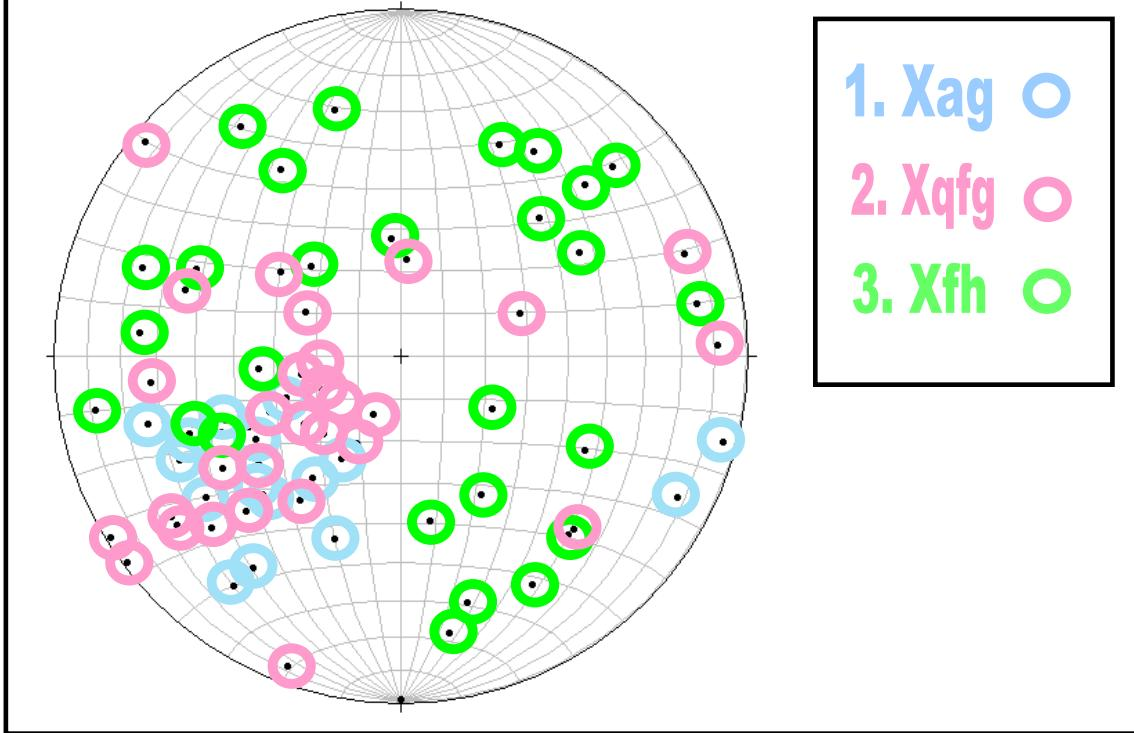
Figure 51. A stereoplot of pole-to-planes for foliations, showing the three broad mappable units. The dispersion in values upridge is thought to be due to greater frost action, measurement of loose blocks of talus/scree or the measurement of unrecognizable limbs of folds (See Figures 56a, 56b, 56e & 56h).
