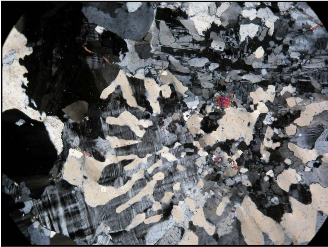
Figure 44e. A photomicrograph of a thin section of an igneous intrusive rock (6.i), showing radiating myrmekitic quartz. Long axis of photomicrograph = 4 mm. (SR1799).
