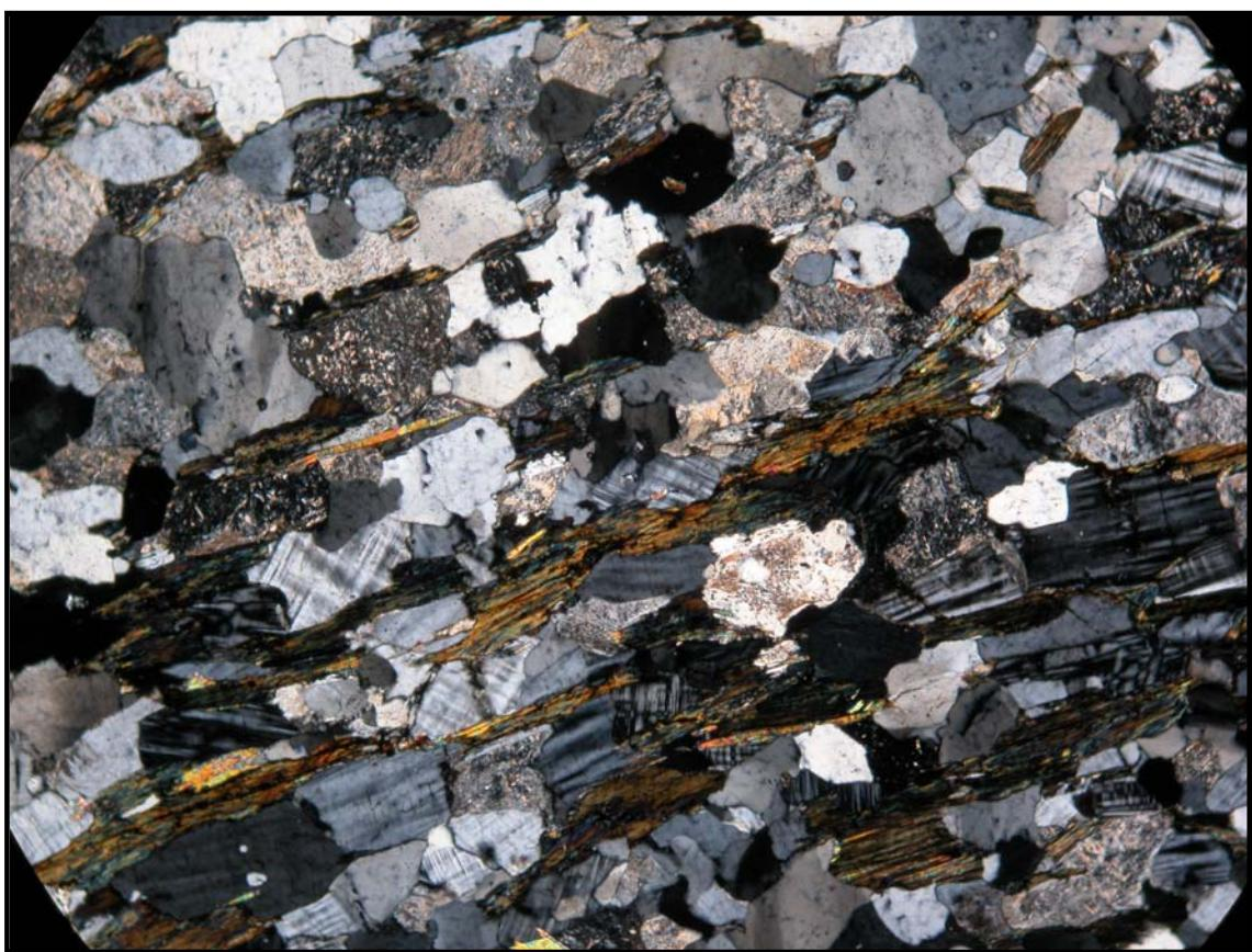
Figure 37c. A photomicrograph of a thin section of Quartzofeldspathic gneiss (2.Xqfg). Long axis of photomicrograph = 4 mm. (NR399).
