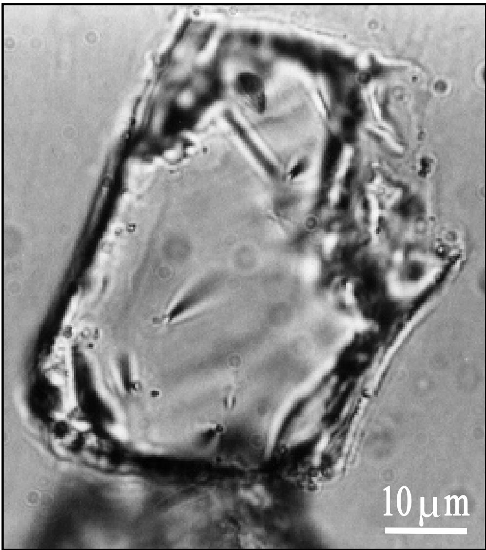
Figure 68. Etched fission tracks confined in the basal plane of an apatite grain observed with oil immersion (etchant: 65%  $HNO_3$  at 20 °C for 15s). 10  $\mu m$  across grain (image courtesy of Shari A. Kelley <http://www.ees.nmt.edu/Geol/Structure/fission.JPG>).
