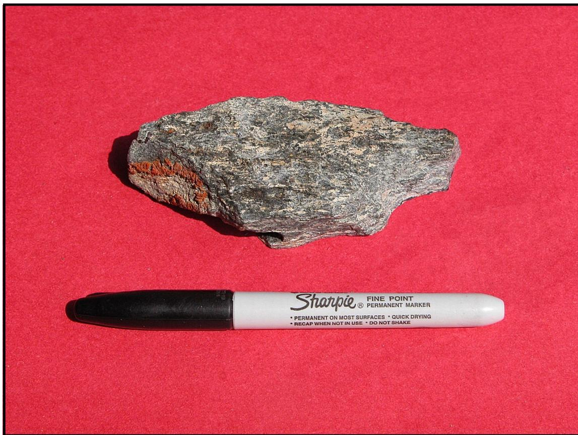
Figure 38g. A hand specimen of feather amphibolite (Xfa) of the felsic hornblendic gneiss (Xfh) unit (3c.Xfh:Xa), showing the weathered gray color. Elongate breakage into shards is also visible. Marker (13.5 cm) is shown for scale. (NR1999)
