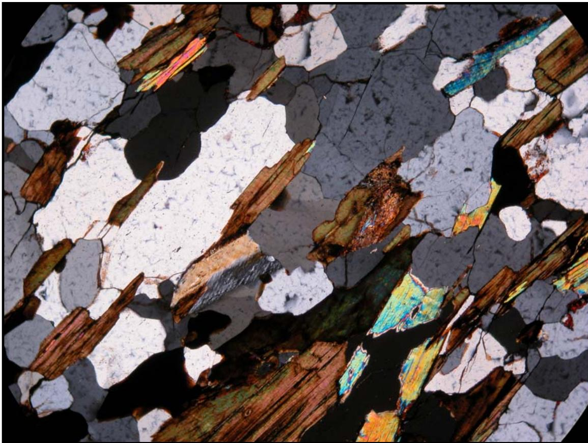
Figure 41c. A photomicrograph of a thin section showing the matrix of the Quartzofeldspathic schist porphyroblastic rock (5b. Pfs). Long axis of photomicrograph = 4 mm. (NR4\*99)
