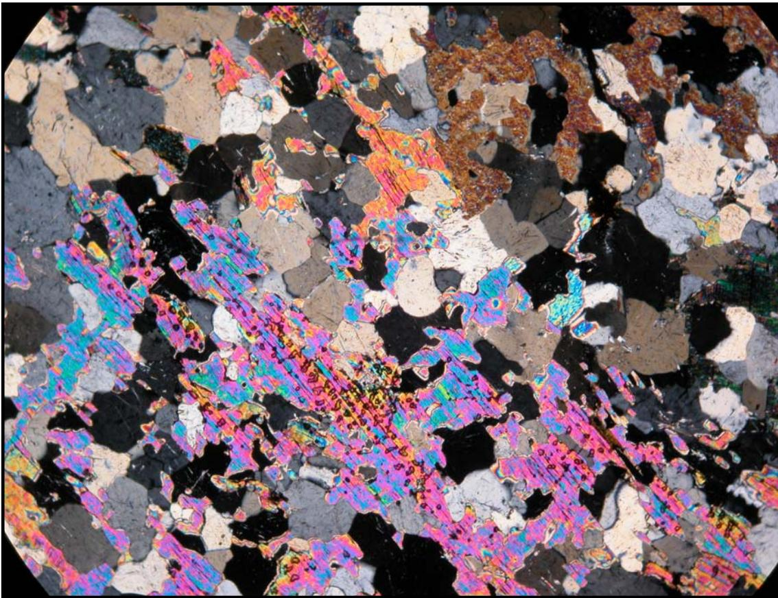
*Figure 40b. A photomicrograph of a thin section of the gray compositionally-banded amphibolite gneiss porphyroblastic rock, showing the quartz and poikiloblastic muscovite within the of porphyroblasts (5a. Pf). Long axis of photomicrograph = 4 mm. (SR3599)*
