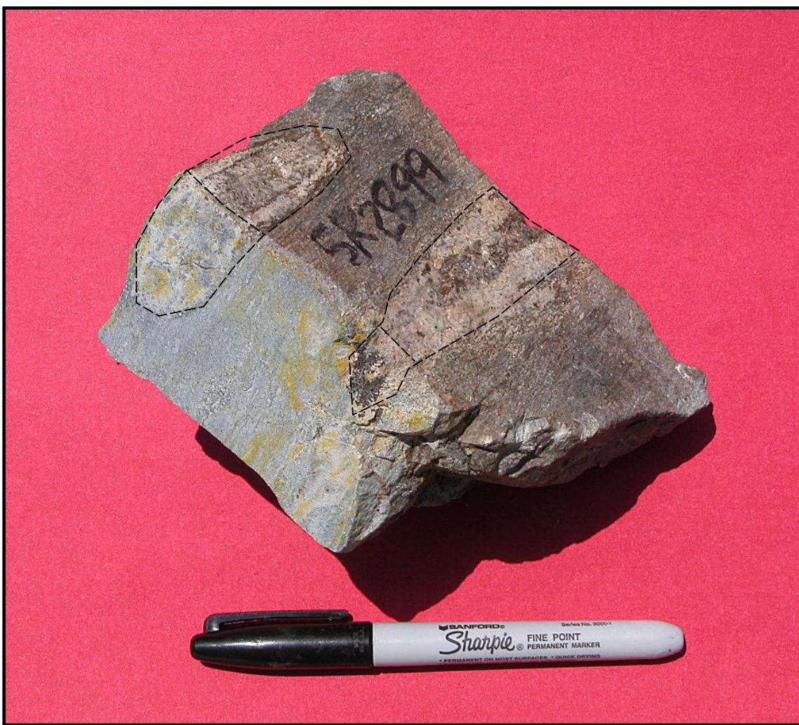
Figure 42b. A hand specimen of the quartzofeldspathic gneiss porphyroblastic rock, showing the porphyroblasts that have been sliced through outlined with a dashed line. Marker (13.5 cm) is shown for scale. (SR2899)
