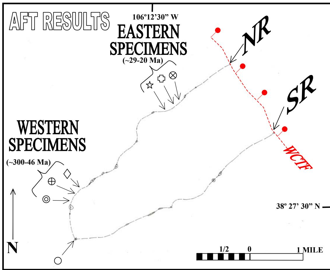
*Figure 73. Simplified Geologic Map showing sample locations along ridgelines relative to the range/basin-bounding fault (WCTF). Refer to Table 4 for sample location symbols and resultant Apatite Fission-Track (AFT) ages.*
