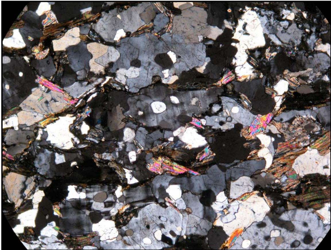
Figure 36b. A photomicrograph of a thin section of the Quartzofeldspathic Schist (Xfs) of the Amphibolite Gneiss (Xag) unit (1c.Xag:Xfs). Long axis of photomicrograph = 4 mm. (NR499).
