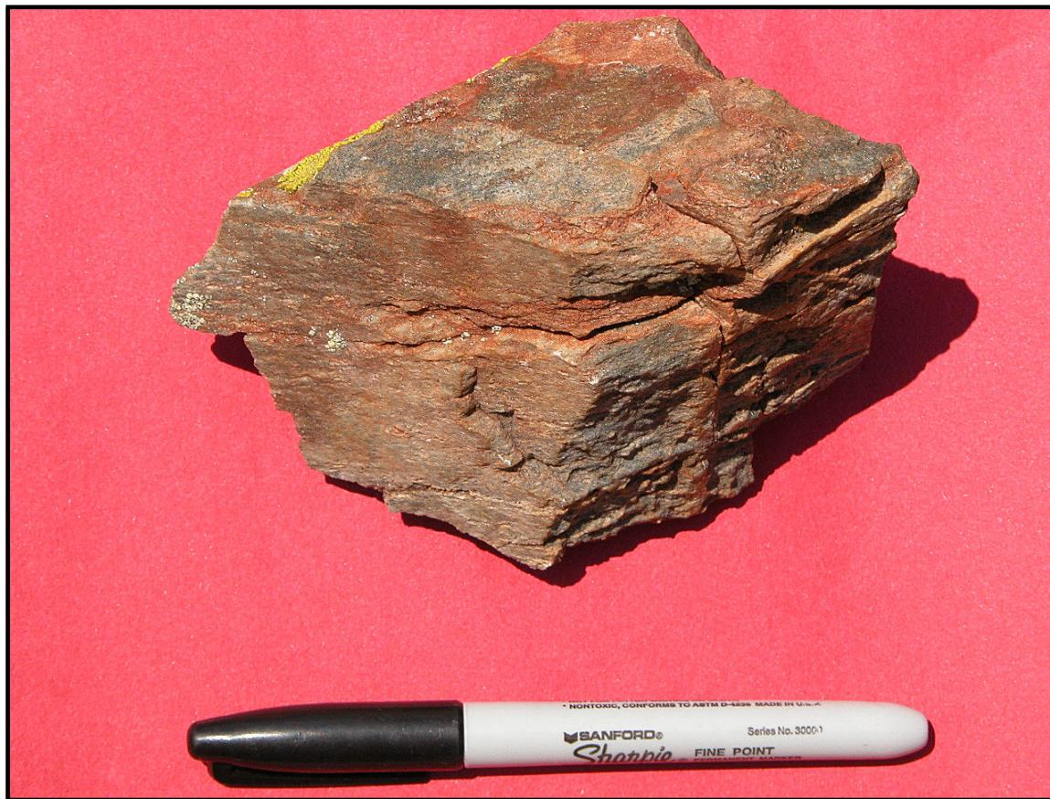
Figure 37b. A hand specimen of Quartzofeldspathic Gneiss (2.Xqfg) showing the orange weathered color. Marker (13.5 cm) is shown for scale. (SR2799)
