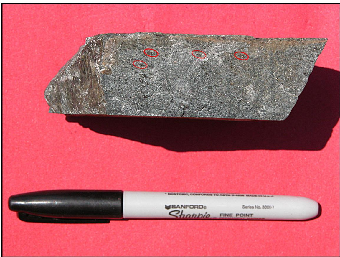
Figure 43a. A hand specimen of hornblende "pods" (outlined in circles) (3d.Xfh:Xhb) in a fine-grained matrix. Marker (13.5 cm) is shown for scale. (NR1399).
