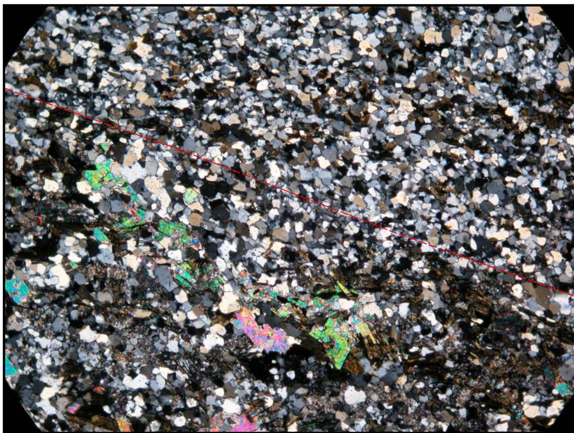
*Figure 42c. A photomicrograph of a thin section of the quartzofeldspathic gneiss “blocks with pods” porphyroblastic rock, showing the pod/matrix contact with a dashed line, with the edge of the porphyroblast in the lower left and the matrix in the upper right of the photomicrograph. Long axis of photomicrograph = 4 mm. (SR2899)*
