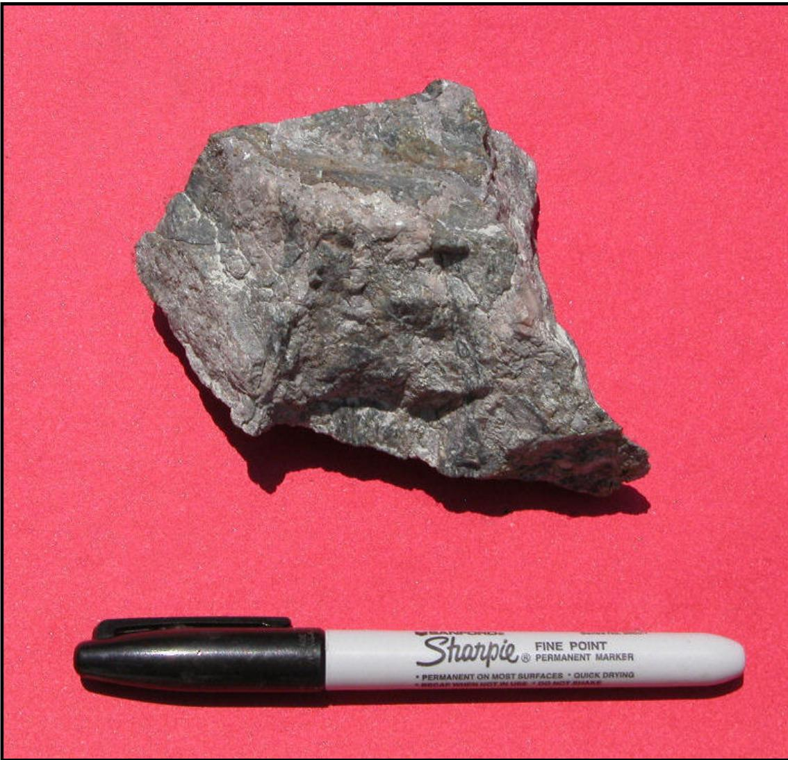
Figure 39b. A hand specimen of a calc-silicate gneiss (4.Xcs (a.k.a 2a.Xqfg:Xcs)), which is exposed within the quartzofeldspathic gneiss (2.Xqfg) unit, showing the fresh color. Marker (13.5 cm) is shown for scale. (NR699).
