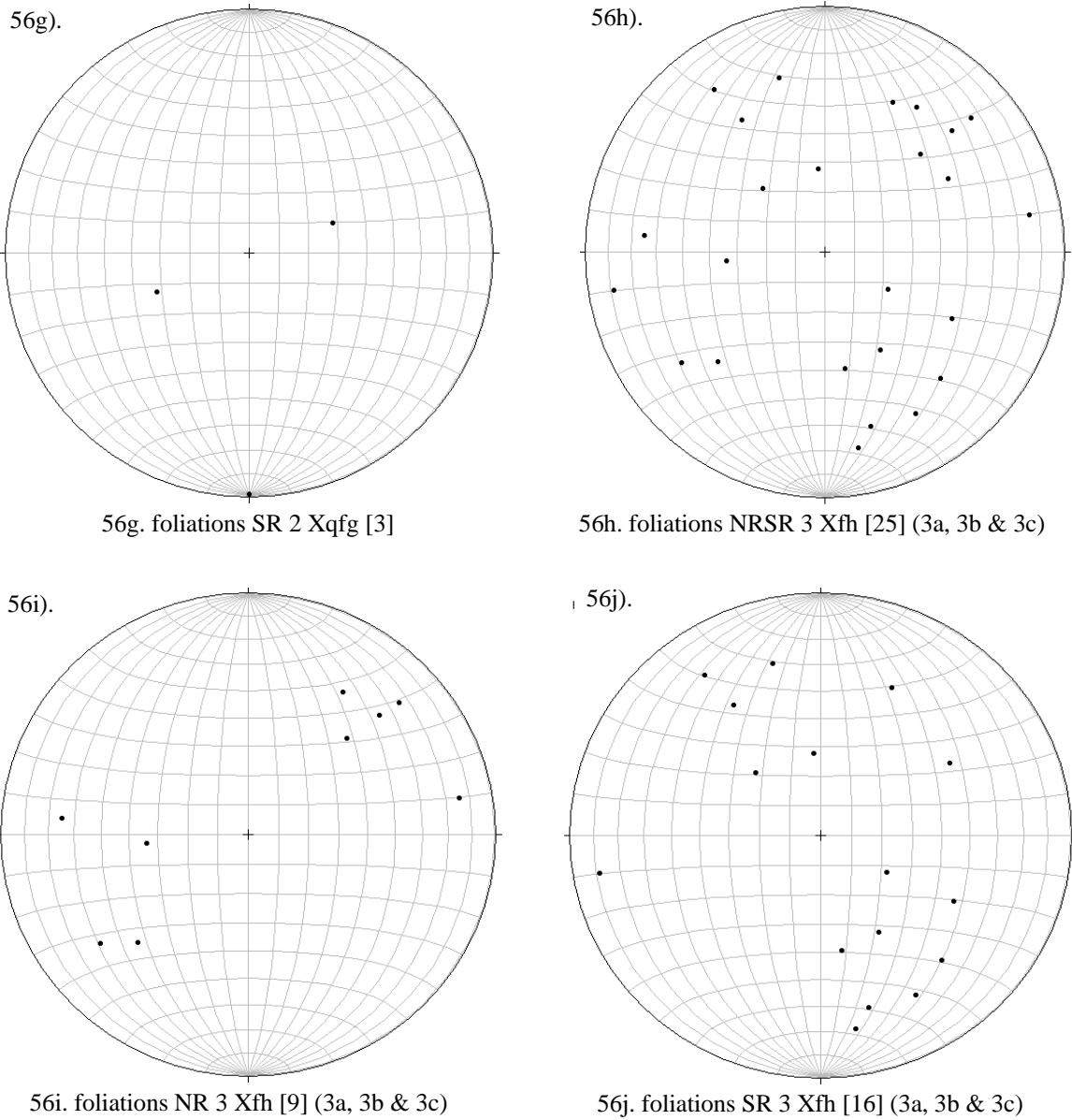
*Figure 56. Lower Hemisphere Equal-Area projected plots (a-j) of field area for metamorphic foliation by both unit and ridgeline.*
