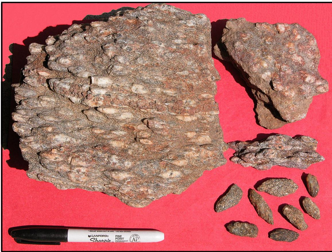
Figure 41a. A hand specimen of Quartzofeldspathic schist porphyroblastic rock (5b. Pfs). Marker (13.5 cm) is shown for scale. (NR4\*99 & SR3799)
