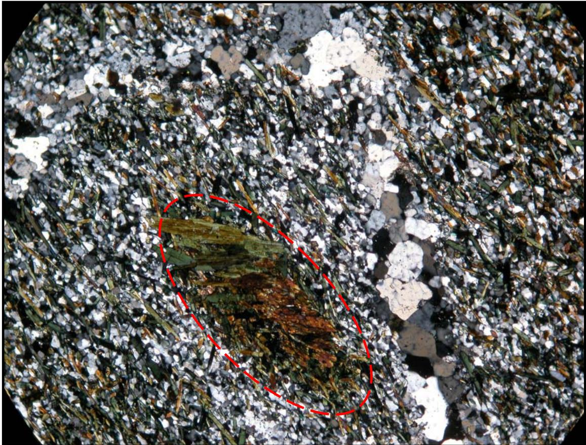
Figure 43b. A photomicrograph of a thin section of a hornblende “pod” outlined by dashed line adjacent to quartz veins. Long axis of photomicrograph = 4 mm. (NR1399).
