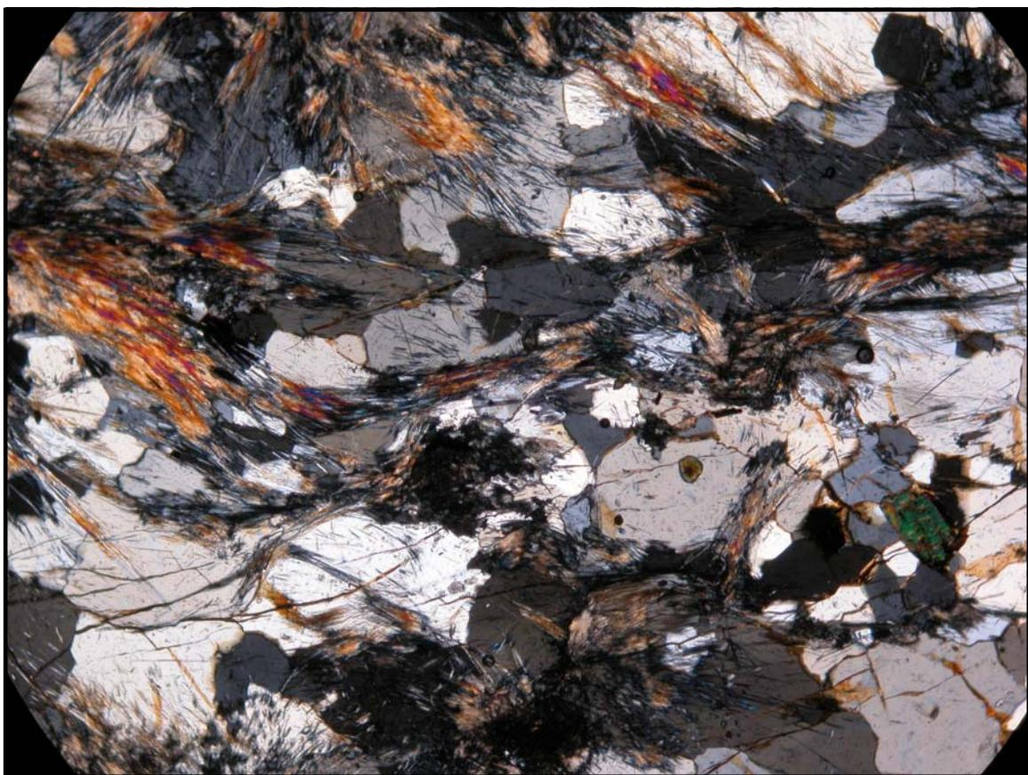
Figure 41b. A photomicrograph of a thin section of the porphyroblasts within the quartzofeldspathic schist porphyroblastic rock (5b. Pfs). Long axis of photomicrograph = 4 mm. (NR4\*99)
