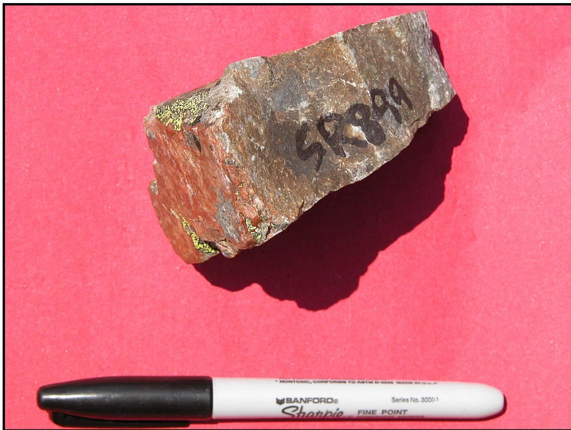
Figure 38e. A hand specimen of a quartzofeldspathic gneiss (Xqf) of the felsic hornblendic gneiss (Xfh) unit (3b. Xfh:Xqf), showing both the weathered and fresh surfaces. Marker (13.5 cm) is shown for scale. (SR899)
