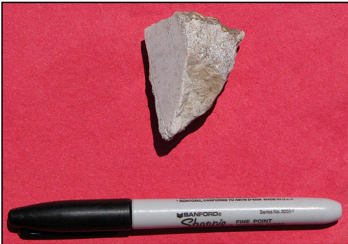
Figure 44f. A hand specimen of quartz mica schist “whiteschist” (3e.Xfh:Xqms). Marker (13.5 cm) is shown for scale. (NR13a99).
