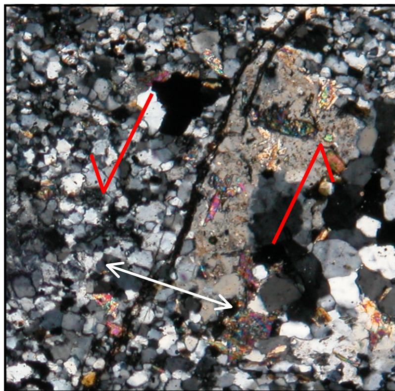
Figure 67b. Close up of fractured and extended grain of NR1099. Long axis of photomicrograph = 0.8 mm.
