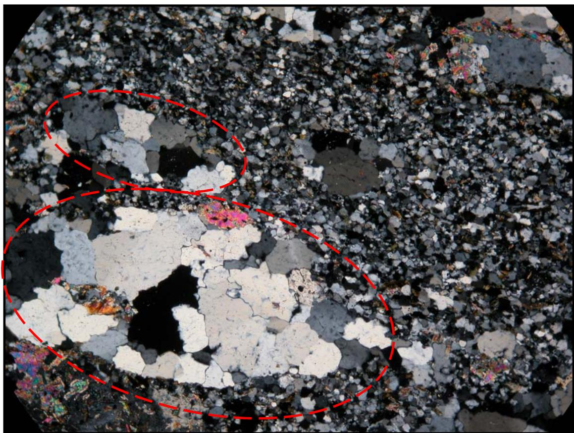
Figure 43c. A photomicrograph of a thin section of the “quartz pods” with the pods outlined with dashed line. Long axis of photomicrograph = 4 mm. (NR1099).
