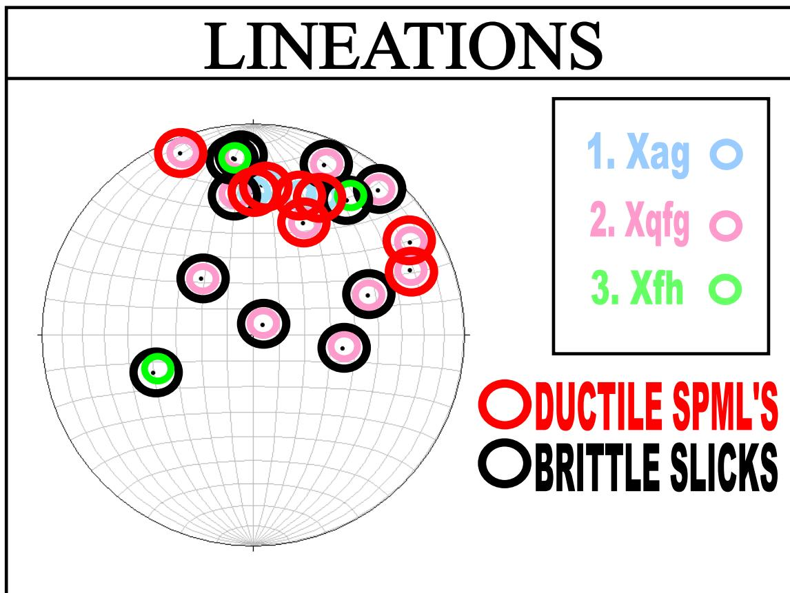
*Figure 52. A stereoplot of pole-to-planes for lineations showing the three broad mappable units and the differentiation between the brittle slickenlines and ductile stretching penetrative mineral lineations (spml's). (See Figures 57a, 57b, 57c and 57d for individual stereonets).*
