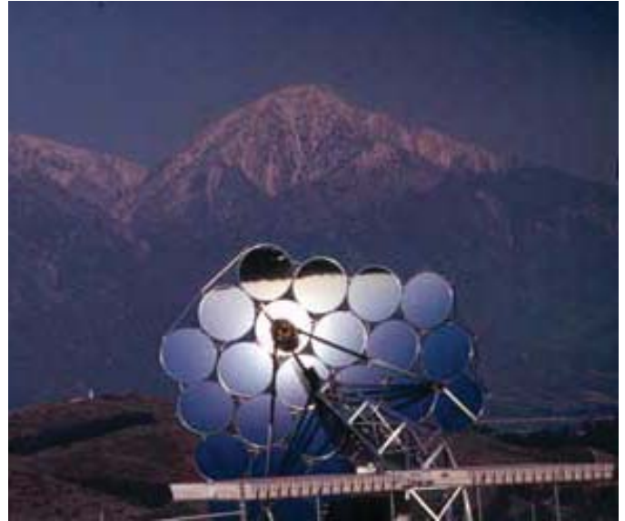
figure 4.37 Dish Stirling solar heat convertor
