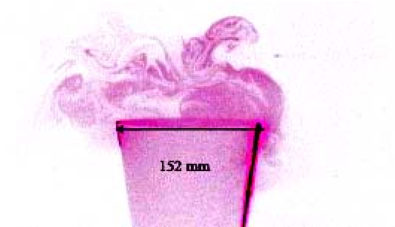
Figure 7-16: Flow visualization using diffuser cone.
