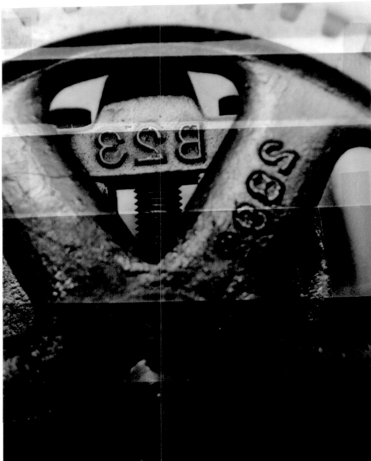
Test Strips of Autoscreen Showing Combinations of Exposures Relating to Over and Under Exposure
