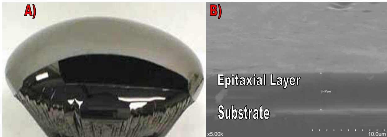
Figure 1.5: A) 4H-SiC single crystal boule produced using the modified Lely process; B) Epitaxial layer grown on 4H-SiC with a thickness of ~5 μm.
