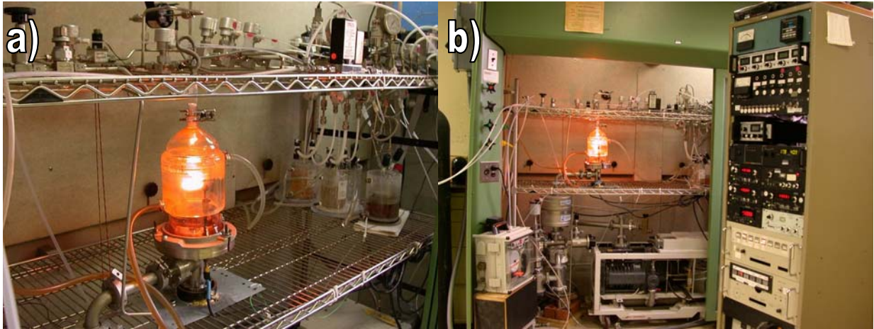
Figure 2.2: Image of the CVD system used for epitaxial growth of SiC, a) Close-up of CVD reactor during epitaxial growth; b) Over view of entire CVD system.
