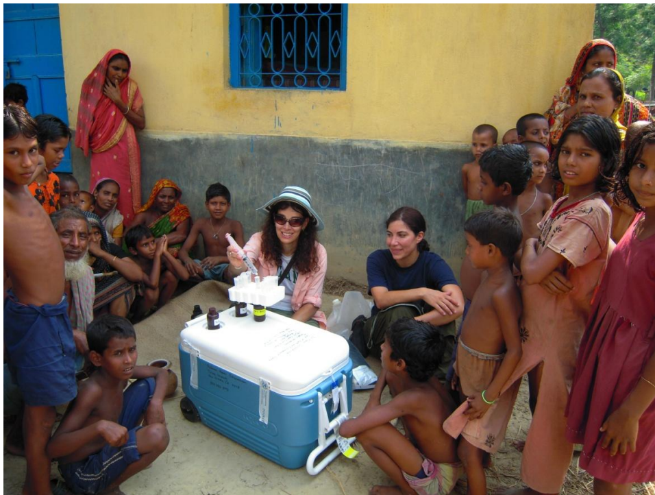
Figure 8: As(III) being separated from As(V) in groundwater samples via anion-exchange columns in Beldanga.
