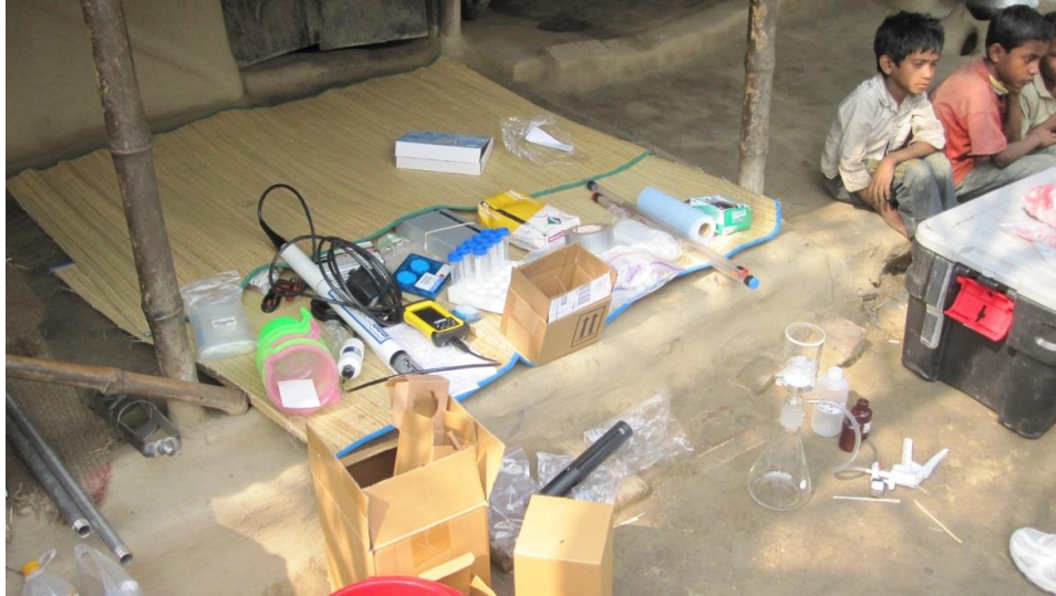
Figure 7: HACH ® Hydrolab ® MiniSonde with hand-held Trimble ® unit, along with other field equipment in Beldanga.
