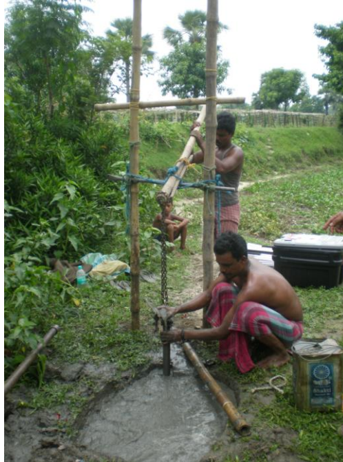
Figure 5: Local drilling method used to collect shallow to deep (< 45 m) sediments in Beldanga.
