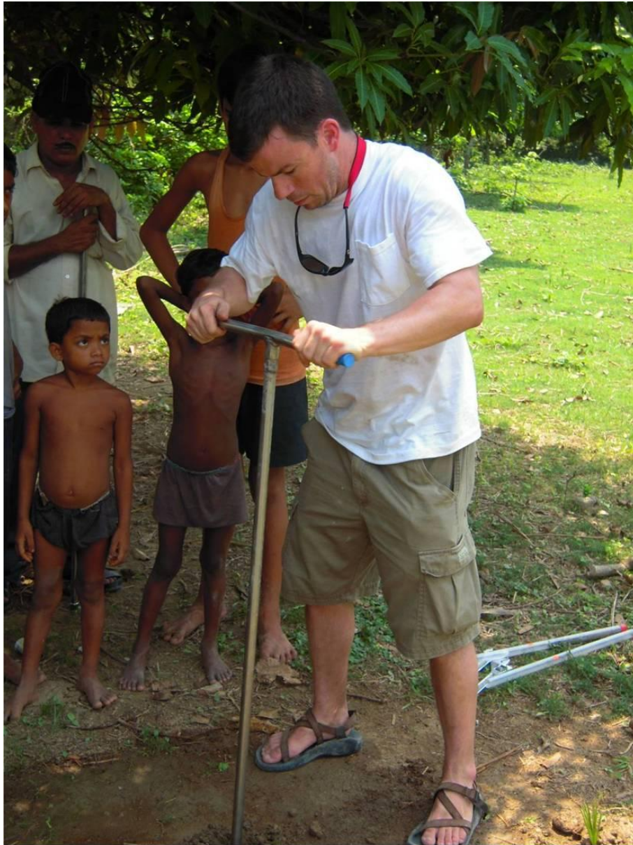
Figure 4: T-handle corer with plastic liner insert being employed to collect surficial (0-2 m) sediments near a tubewell in Hariharpara with significantly elevated concentrations of dissolved As.
