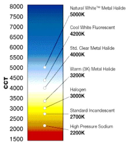
**Figure 3-4: Graphic of color temperature of common light sources.**
