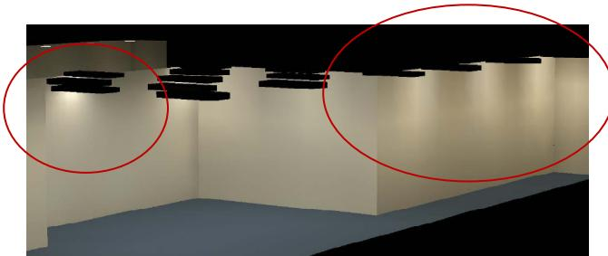
**Figure 6-6 Rendering of recessed fluorescent fixtures**
