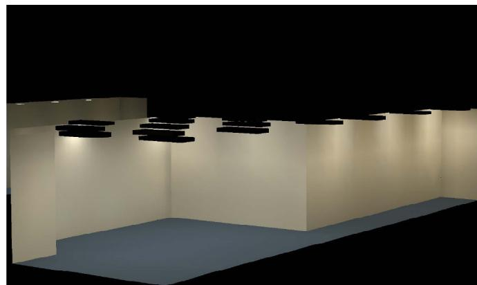
**Figure 6-2:** AGI32 rendering of recessed 2 x 4 troffer fixture layout for a typical classroom.
