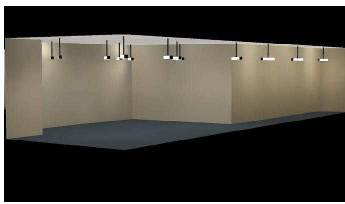
**Figure 6-3:** AGI32 rendering of suspended indirect/direct fixture layout for a typical classroom.
