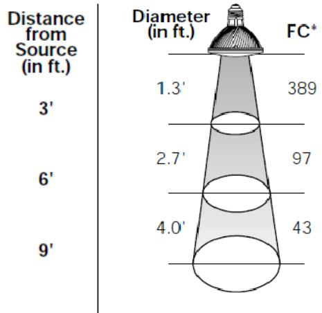
**Figure 6-4 Conic distribution of light from a 60W PAR 30 normal flood lamp.**
