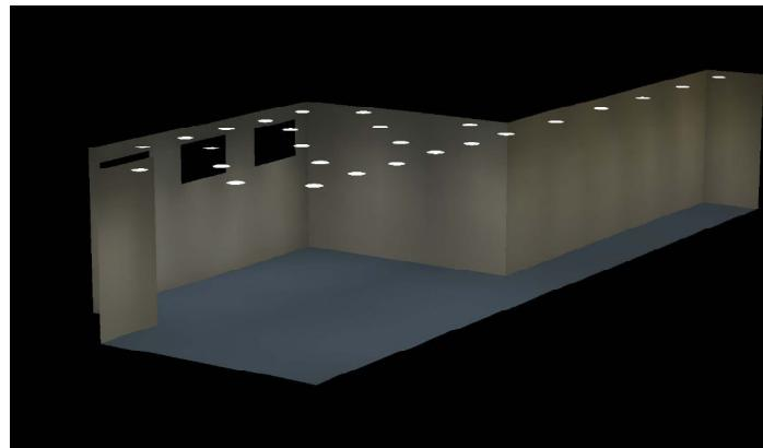
**Figure 6-1:** AGI32 rendering of incandescent fixture layout for a typical classroom.
