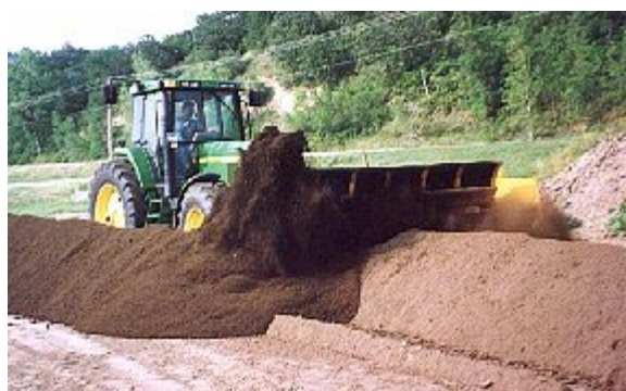
FIGURE 2. The PTO PA35C-10.5 compost turning unit is designed to be attached to the front of 100-160 HP farm tractors (Brown Bear Corp., 2003).
