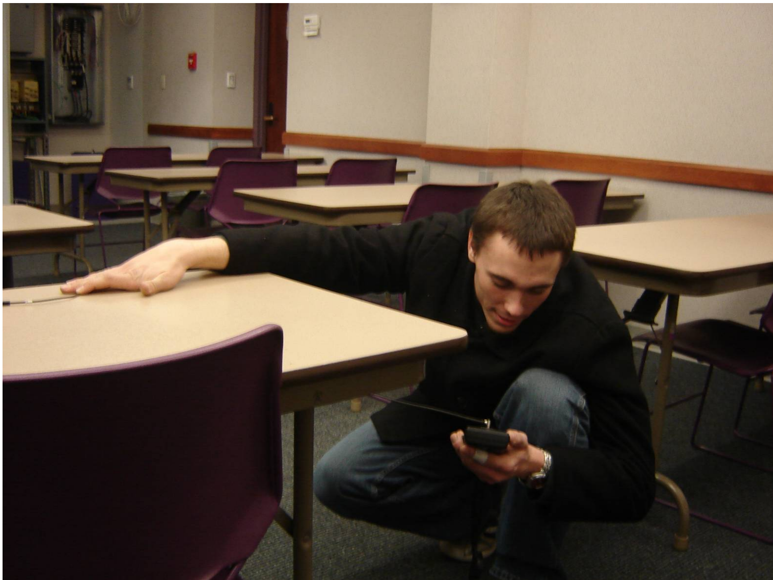
Figure C.5 Robert Nelson properly taking a footcandle reading on the task plane
