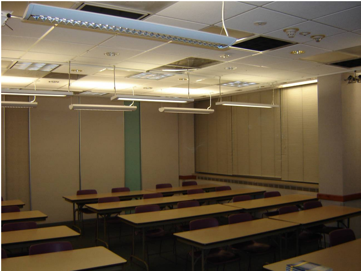
Figure 3.4 30fc Uniform Lighting Lab Mockup
