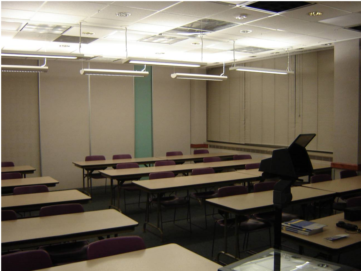
Figure 3.2 50fc Uniform Lighting Lab Mockup
