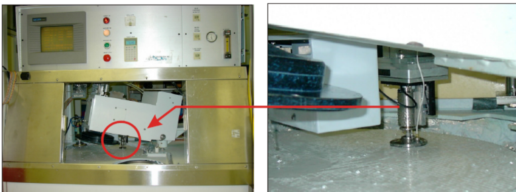
Figure 2.10 PadProbe™ Installed in a Polisher [Center for Tribology Inc., 2006]
