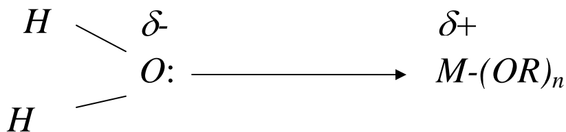
Figure 1.4 Nucleophilic attack of water on the metal center in a metal alkoxide ( M-(OR)_n ) where M : metal and R : alkyl group
