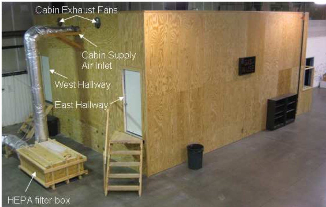
Figure 2.1: Chamber Exterior, Inlets, and Exhaust Fans
