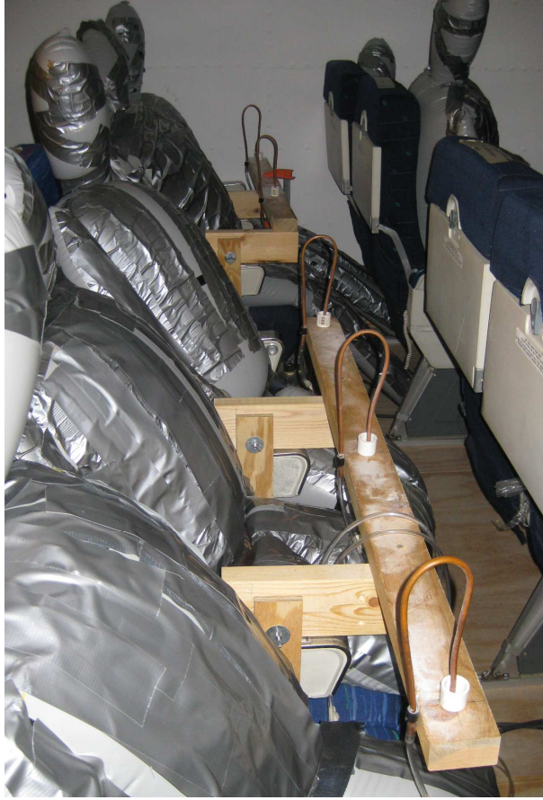
Figure 2.23: Particle Dispersion System in Row 2
