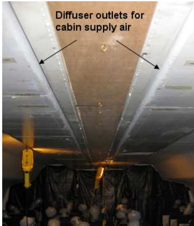
Figure 2.9: Cabin Diffuser Outlets
