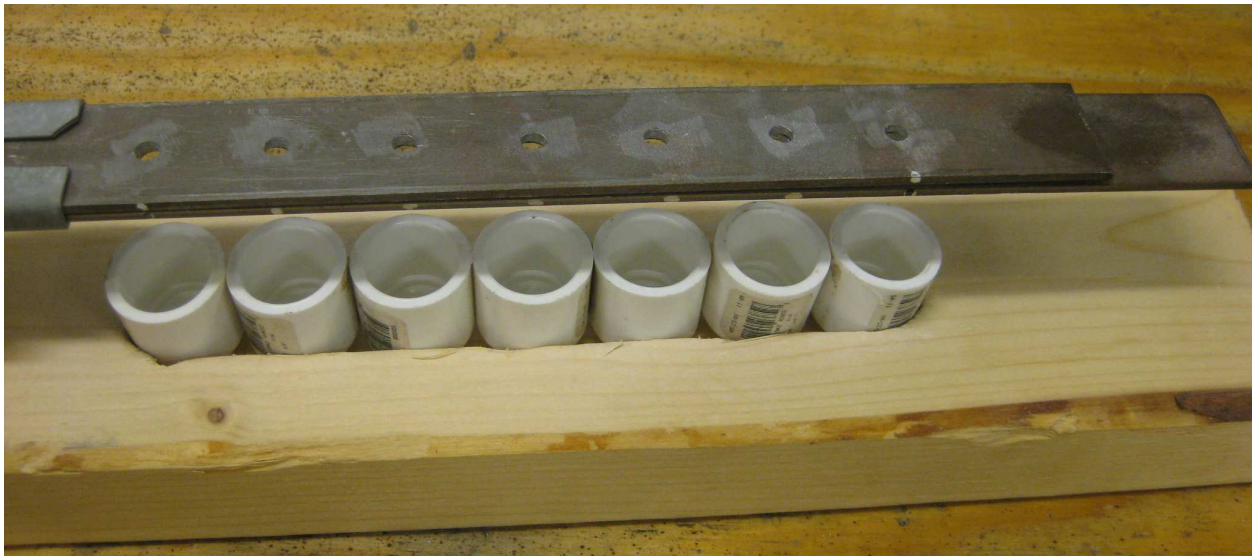
Figure 3.1: Measurement Plate and Tray for Pre-Test Cap Loading
