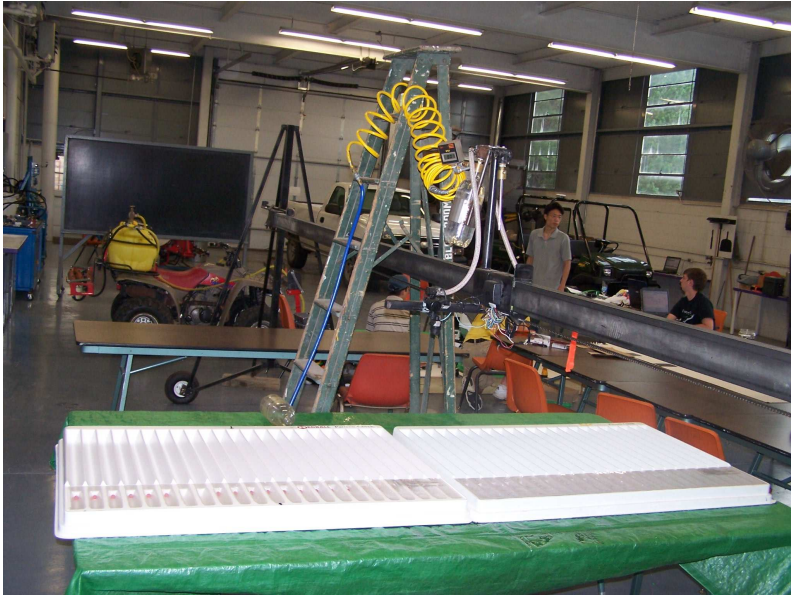
Figure 3.16 Pattern check was placed such that the center of the nozzle matches the center of pattern checks
