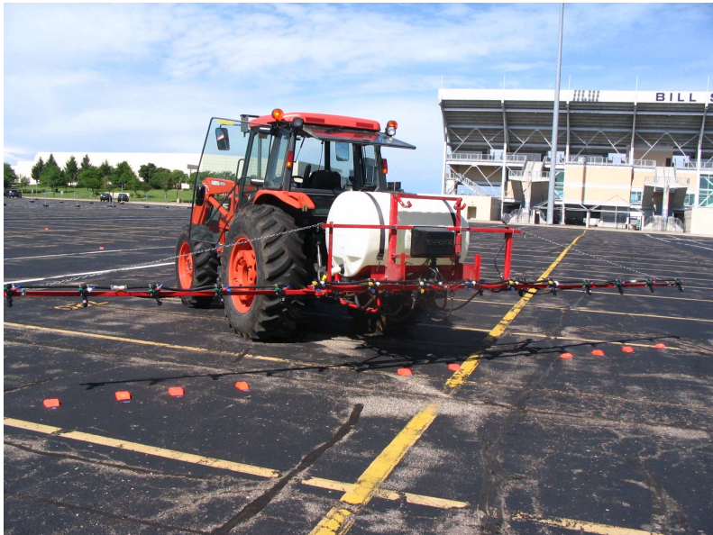
Figure 4.2 Sprayer with 25ft boom attached to the tractor and ready for spraying
