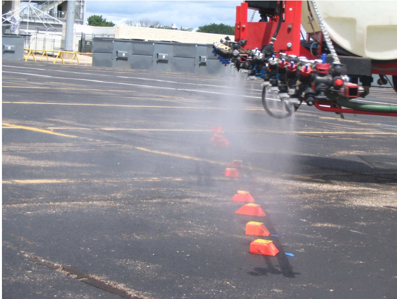
Figure 4.3 Sprayer spraying on water sensitive cards
