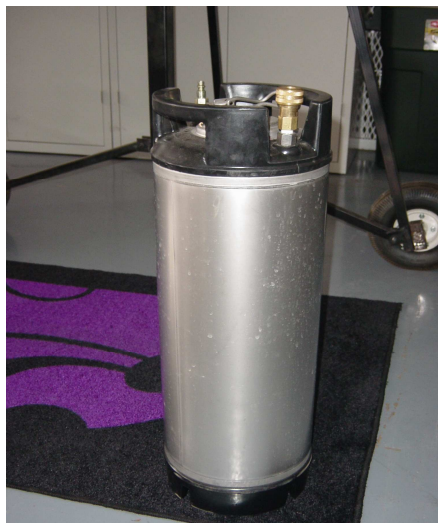
Figure 3.6 Five gallon pressurized steel container with spray adapter and air adapter
