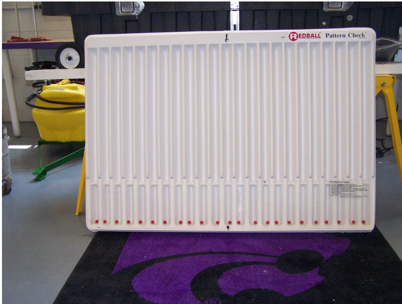
Figure 3.13 Pattern check used for measuring uniformity of spray distribution
