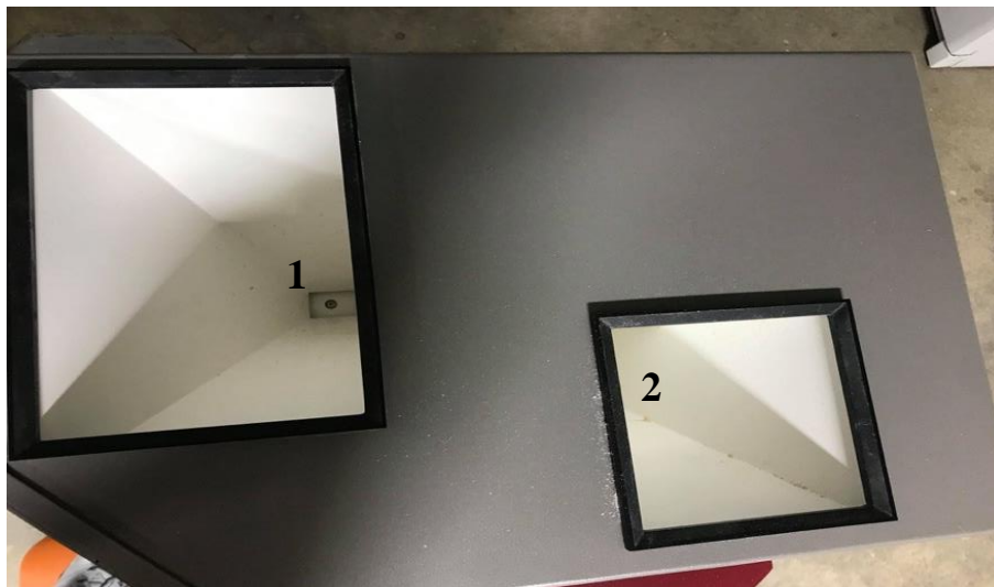
Figure 3.2 Hopper surface of the lab mill; 1 - BK hopper and 2 - RD hopper
