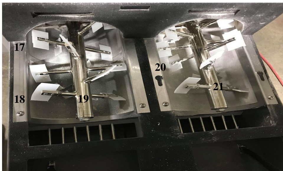
Figure 3.6 SZ and RD Sifter system; 17 - SZ flour sifter, 18 - FM sifter, 19 – SZ beater paddle (n = 2), 20 - RD flour sifter, and 21 - RD beater paddle (n = 2)
