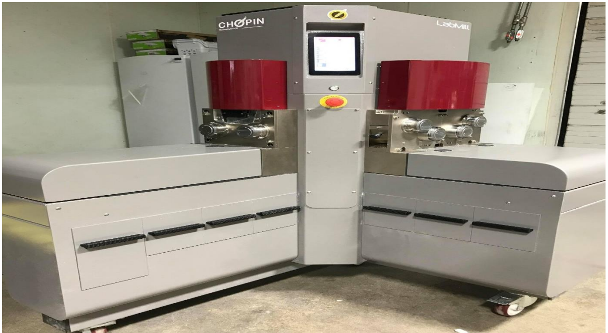
Figure 3.1 Chopin (Chopin, France) lab-scale roller mill used in the milling experiment
