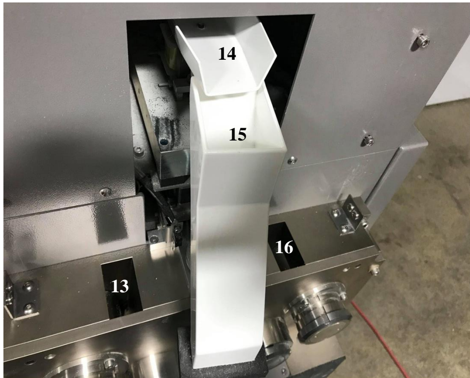
Figure 3.5 SZ and RD system; 13 - SZ roll, 14 - RD feeder, 15 - RD feeder guide, 16 - RD roll
