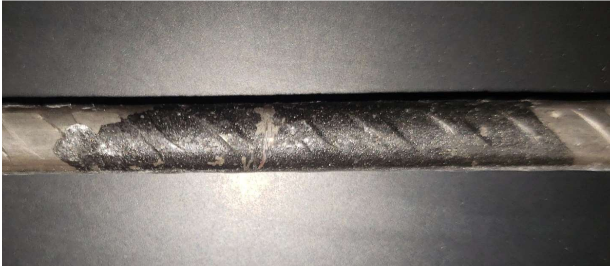
Figure 7.18 Typical mark from wire scriber
