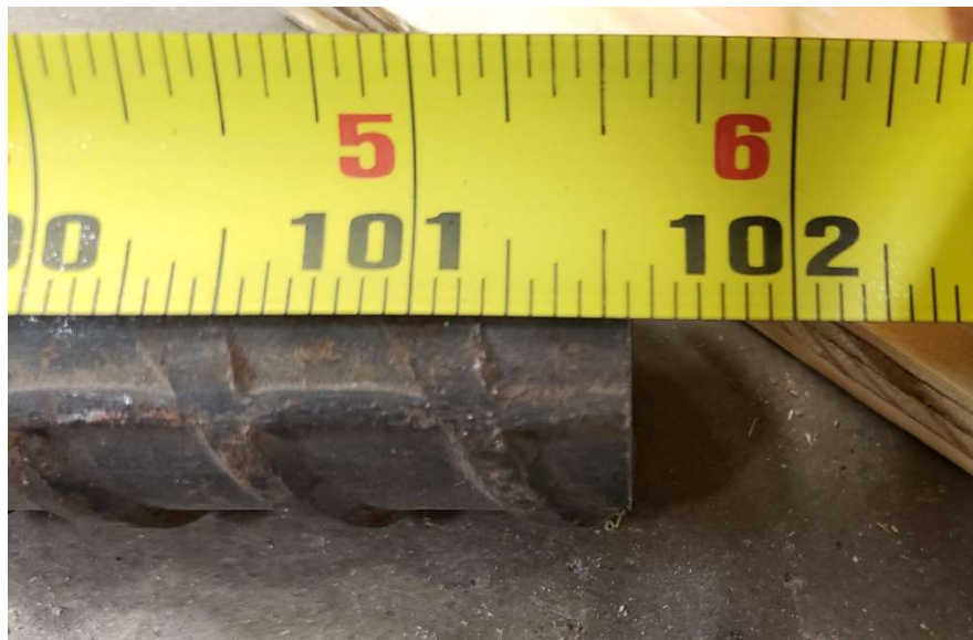
Figure 7.3 Length of rebar used as gage block
