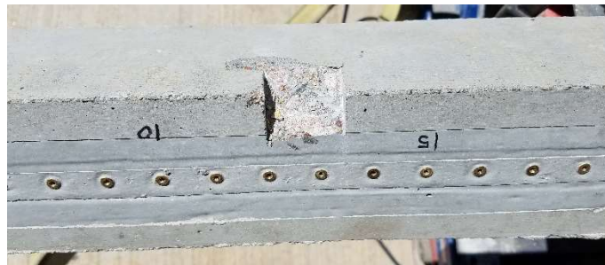
Figure 5.4 Typical groove in prism
