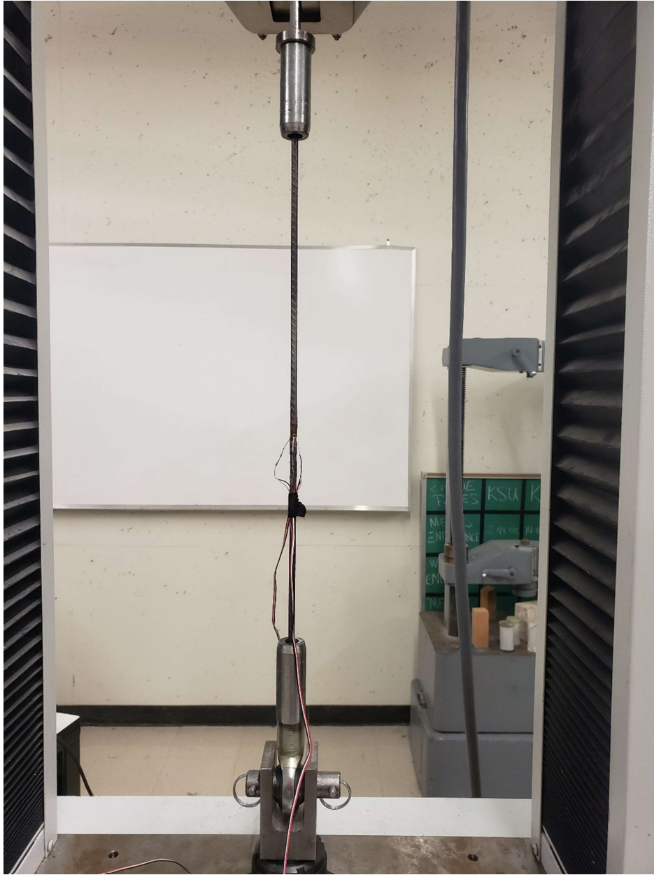
Figure 6.18 Wire bow test setup
