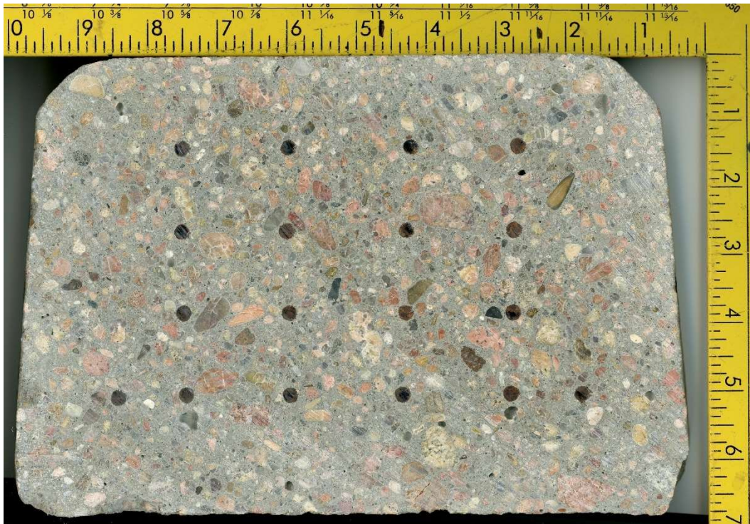
Figure A.10 Typical mid-span cross-section of tie type E
