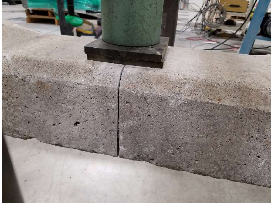
Figure 5.15 Notch cut at mid-span of tie D4
