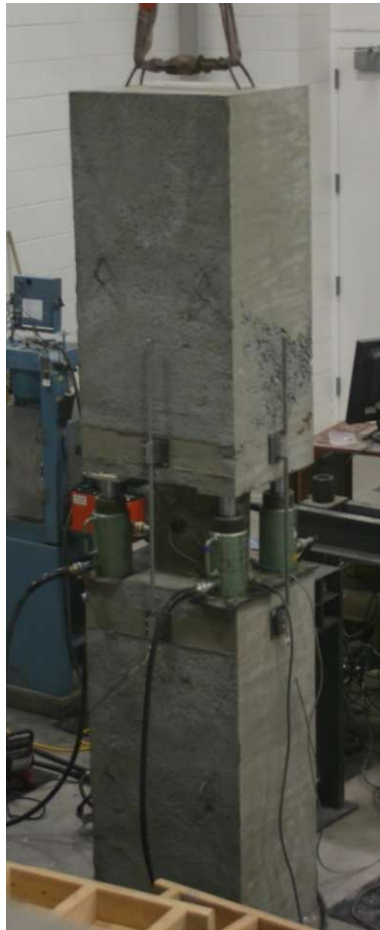
Figure 5.25 Test configuration for tension test
