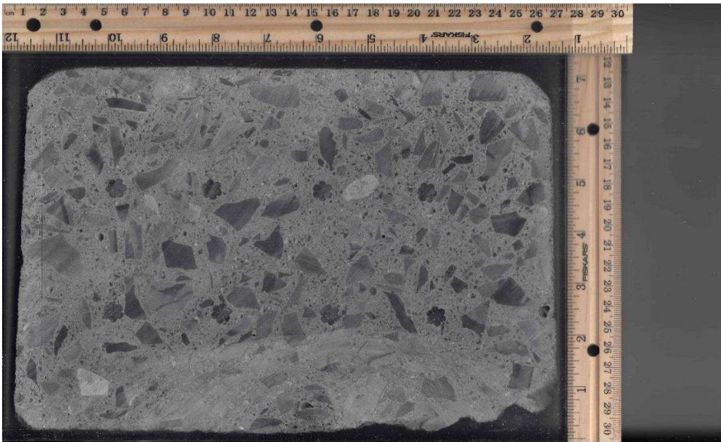
Figure A.14 Typical mid-span cross-section of tie type G
