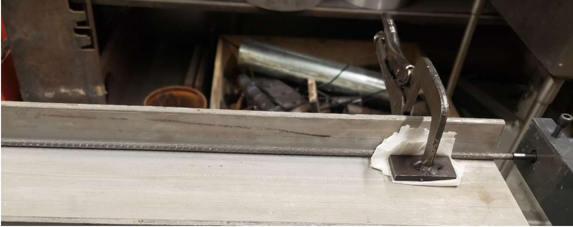
Figure 7.12 Clamping used to keep wires straight
