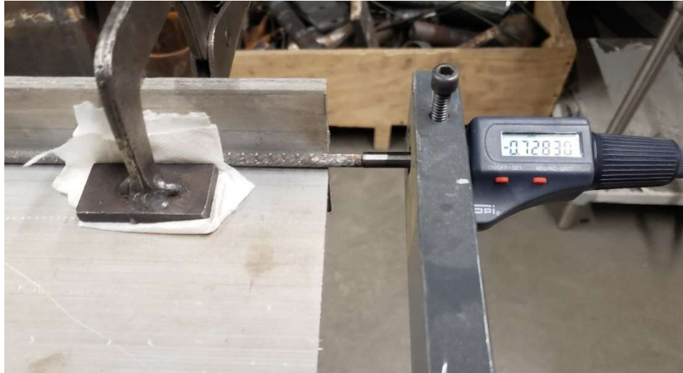
Figure 7.14 Micrometer centered on wire
