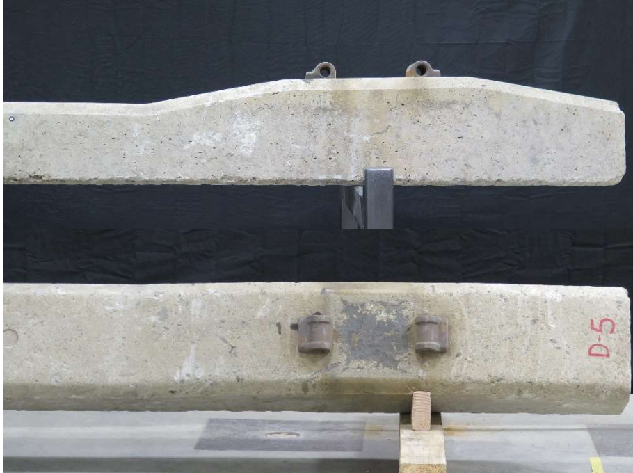
Figure A.7 Typical side and top view of tie type D
