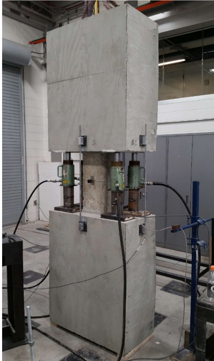
Figure 5.20 Test configuration for preliminary tie test
