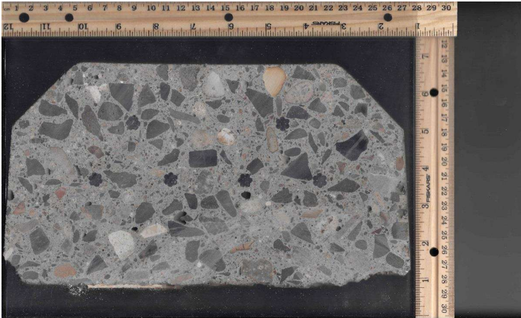
Figure A.6 Typical mid-span cross-section of tie type C
