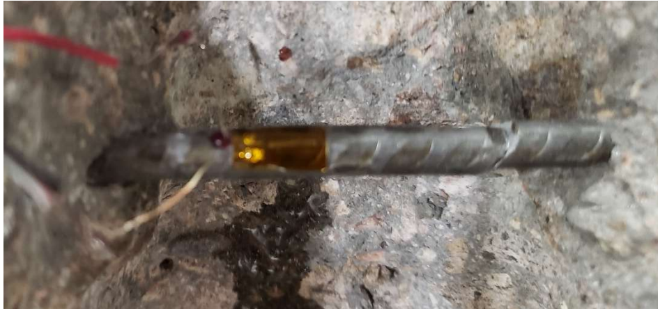
Figure 6.12 Wire in bent position after cutting
