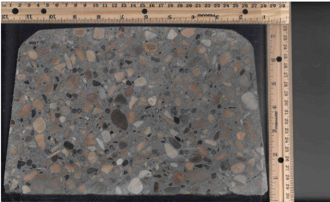
Figure A.20 Typical mid-span cross-section of tie type K
