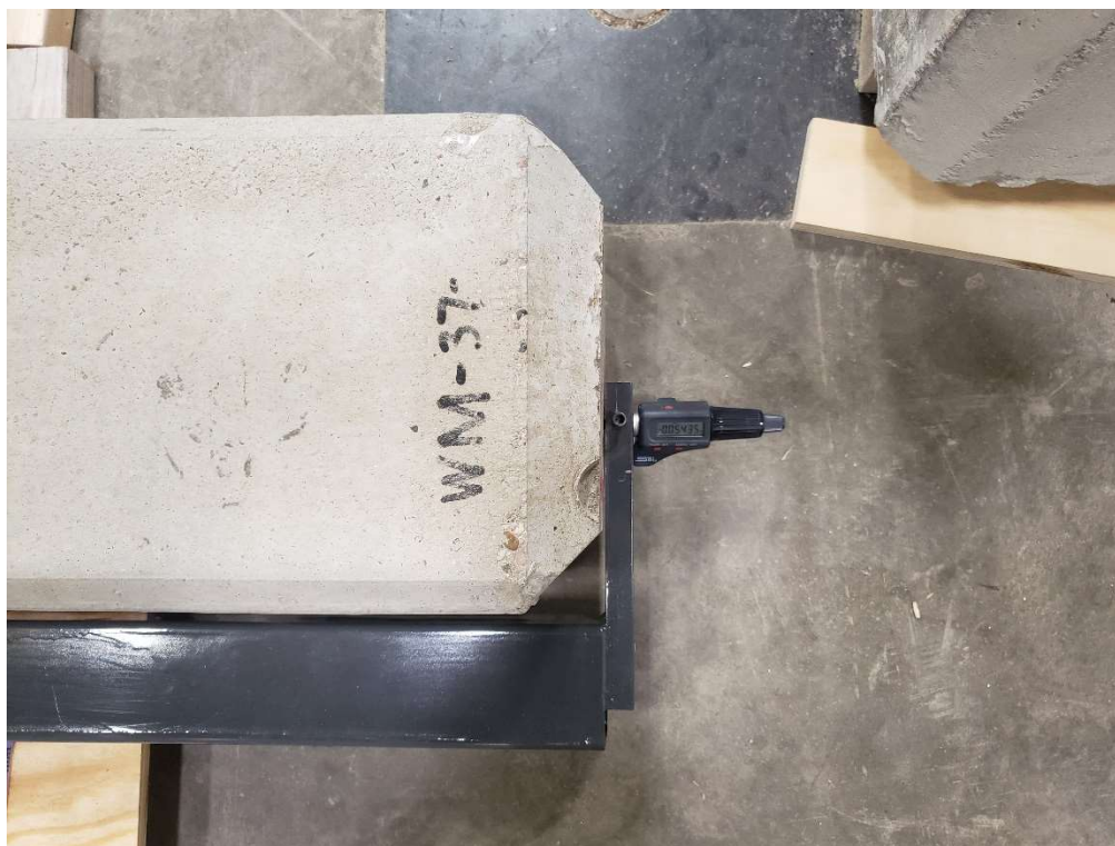
Figure 7.8 Micrometer measuring wire length
