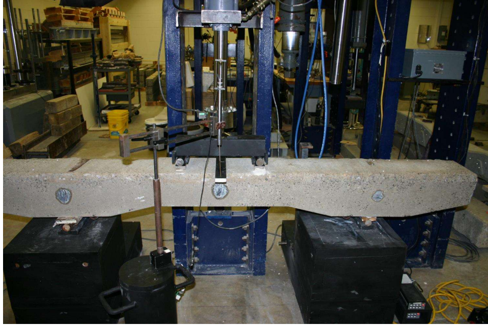
Figure 8.2 Flexural test setup
