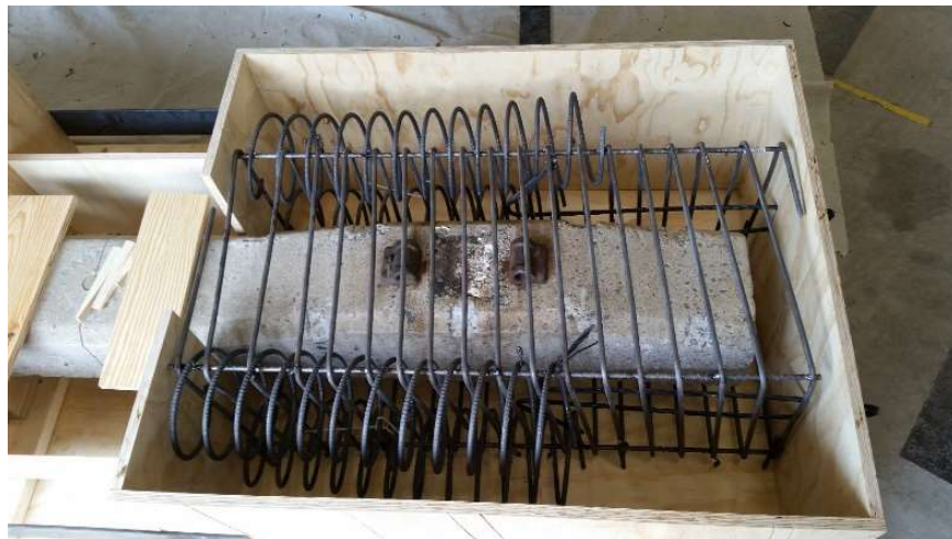
Figure 5.18 Rebar caging used for preliminary tie testing
