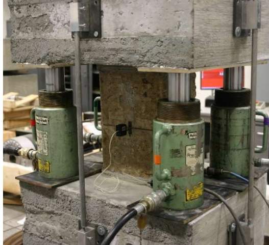
Figure 5.26 Typical instrumentation configuration for tension test
