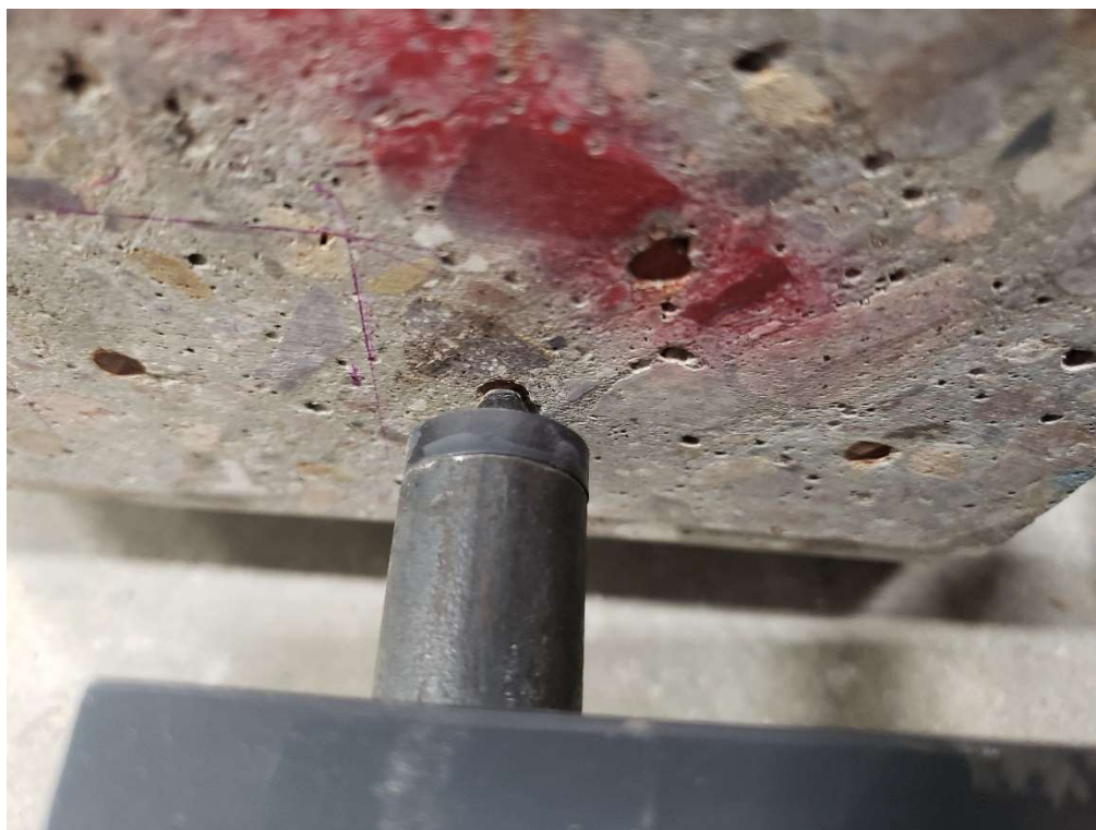
Figure 7.7 Conical piece centered on the end of a wire
