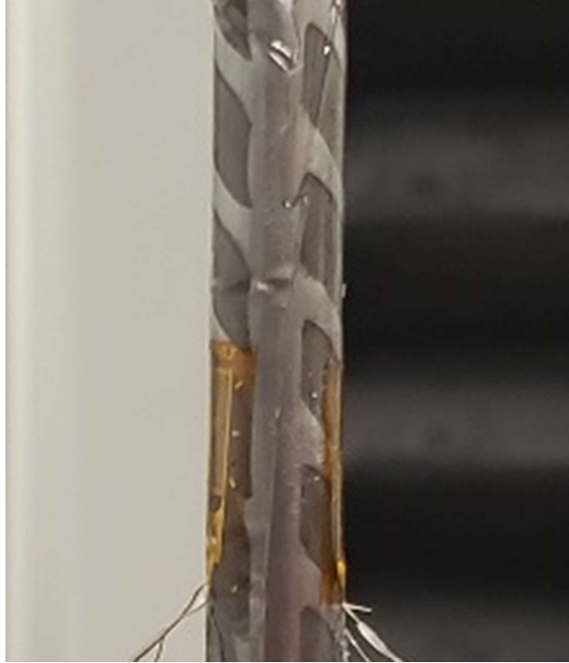
Figure 6.19 Strain gages instrumented on opposite faces of wire
