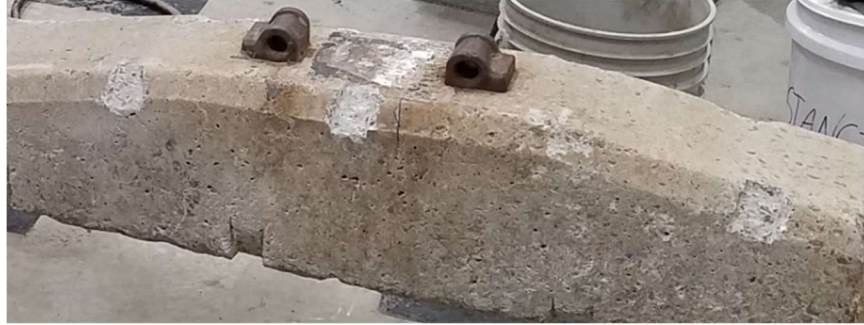
Figure 5.17 Grooves added at ends of tie
