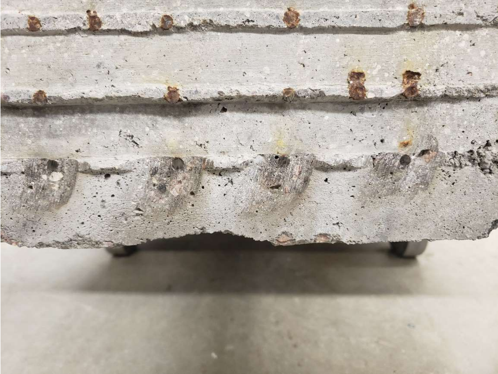
Figure 7.4 Smoothed wire surfaces for length measurement
