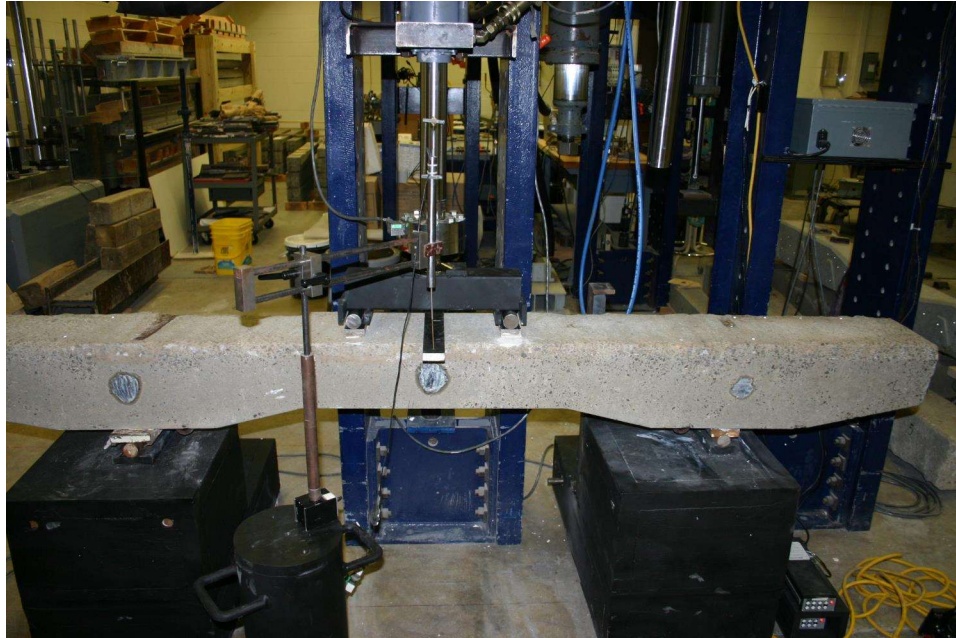
Figure 4.2 Typical flexural configuration
