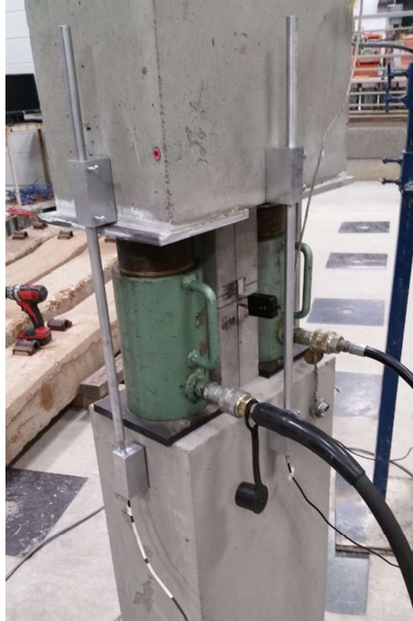
Figure 5.8 Test configuration for prism testing
