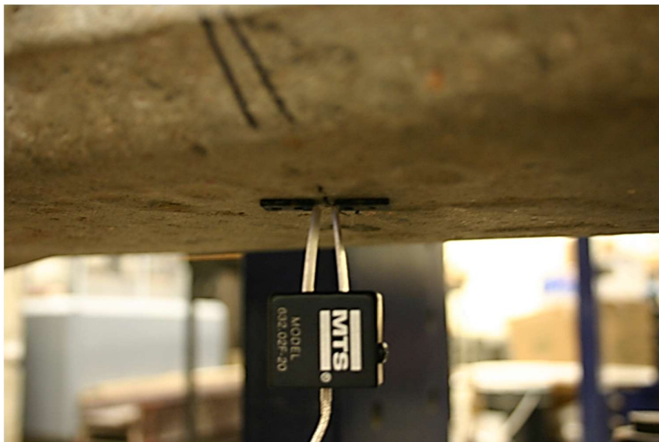
Figure 4.3 Clip gage instrumented over crack
