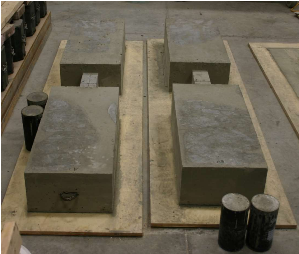
Figure 5.6 Prisms after casting blocks
