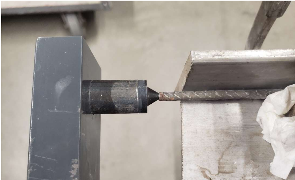
Figure 7.13 Conical end piece centered on wire
