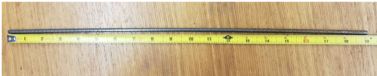
Figure 6.16 Bow in unstressed wire
