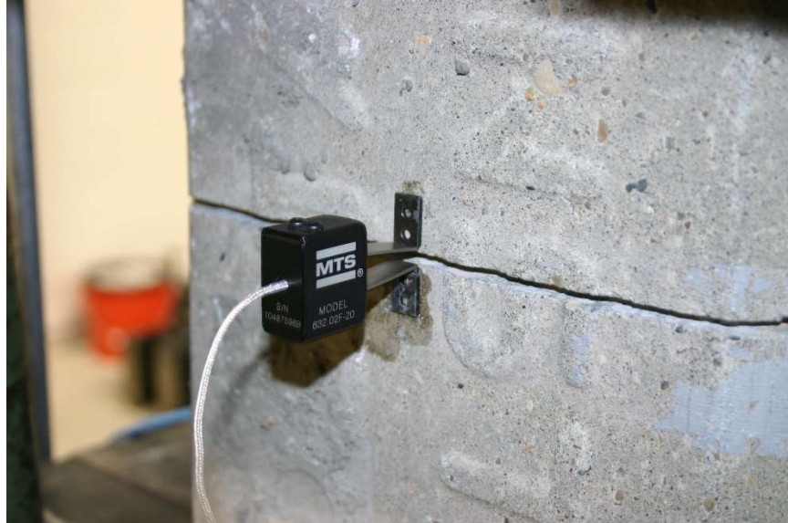
Figure 5.19 Clip gage instrumented over the notch
