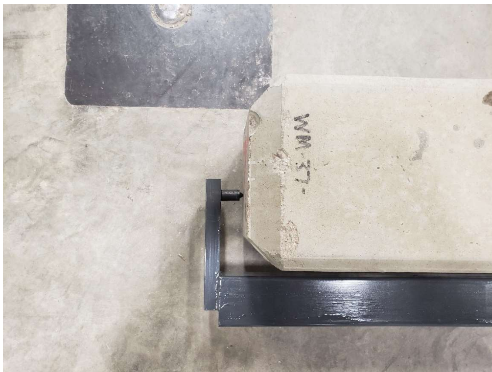
Figure 7.6 Conical end piece at end of tie
