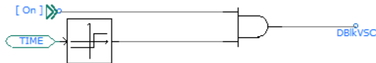
Figure A.4 Inverter Startup Sequence Circuit Diagram in PSCAD
