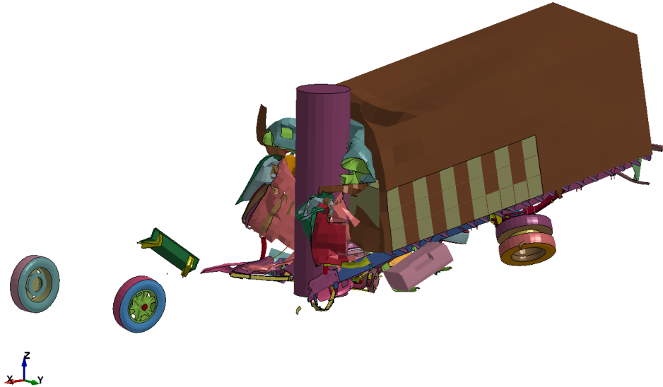
Figure 3.6: F800 and semi-rigid column at 0.174 seconds after impact
