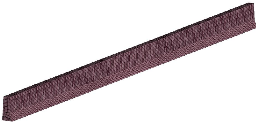
Figure 3.17: Concrete barrier mesh as modeled for transient dynamic simulations
