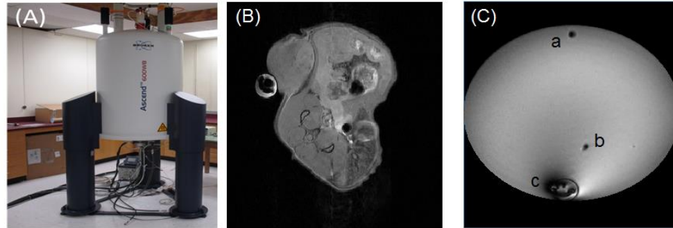
Figure 2.14 (A) Photograph of a vertical MRI scanner, (B) in vivo anatomical image of mouse, (C) tissue-mimicking phantom, a and b are fiber optic temperature probes inserted inside the phantom to validate the temperature measurement with PRFS method and c shows the heating applicator
