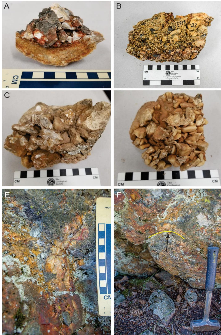
Figure 3.4: Rock sample images of clast-supported breccia and field images of silica infiltrate. A) Portion of clast-supported breccia that has fallen onto the sinter bed that at the time existed as a silica gel, thus deforming it upon impact. B-D) Clast-supported breccia with varying clast sizes cemented together by a final coating of sinter. E-F) Silica infiltrate (highlighted by yellow line and arrow) taking advantage of pre-existing cracks in the underlying host rock. Image E is rotated 90° from horizontal.
