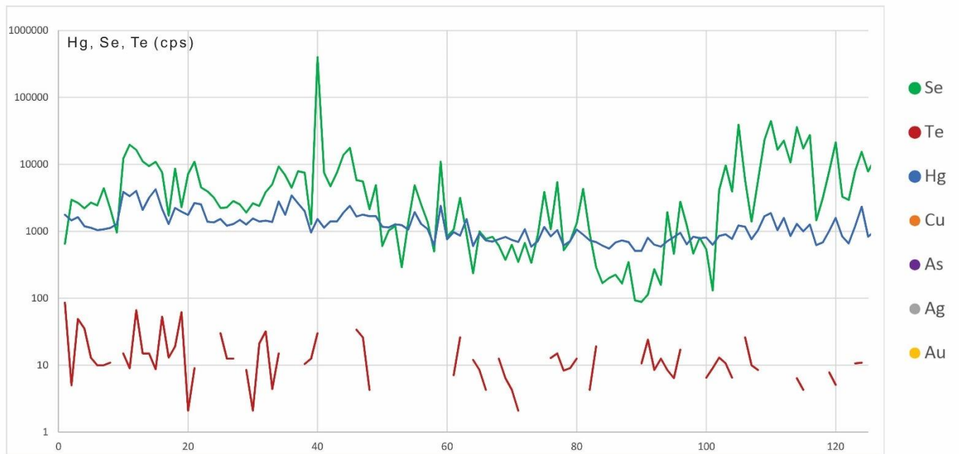
Figure 3.19: LA-ICP-MS transect of mid-slope apron sample EF19-5 (middle) and data in ppm (above) and cps (below).
