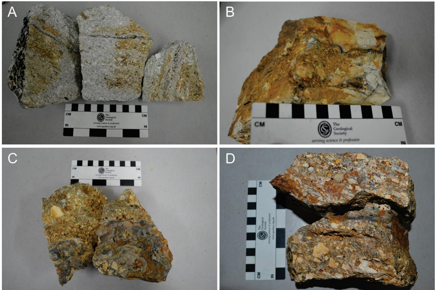
Figure 3.3: Matrix-supported breccia found on the Main Knob at Milestone. Unsorted grain sizes range from ~0.1-8 cm. Matrix consists of white, gray, tan, or black sinter, with fine (~0.3 cm) interbedded layers of laminated sinter. A) Matrix supported breccia consisting of gray-colored sinter matrix with white argillically-altered rhyolite clasts (up to ~2 cm) and a single layer of interbedded black sinter. B) Light-tan matrix breccia with an oxidized surface containing large clasts (~8 cm) of argillically-altered country rhyolite. C) Matrix-supported breccia with overlying dark-gray/black sinter. D) Gray matrix breccia with unsorted clasts and interbedded black sinter overlying the breccia.
