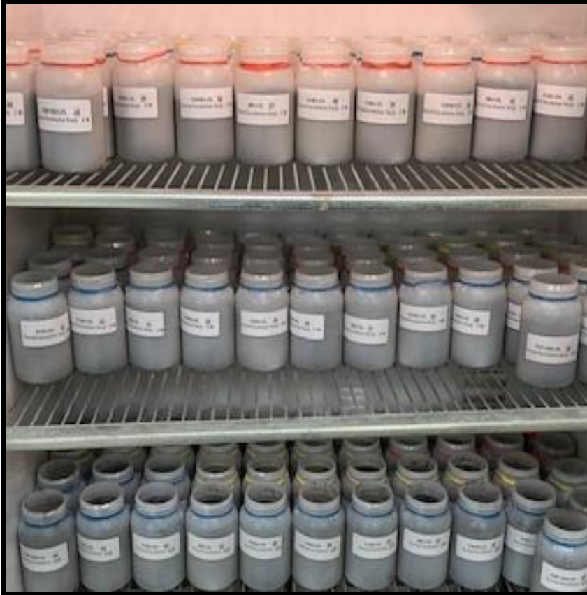
Figure C.1 Incubation study samples incubated at a controlled temperature incubator maintained at 25°C for six months
