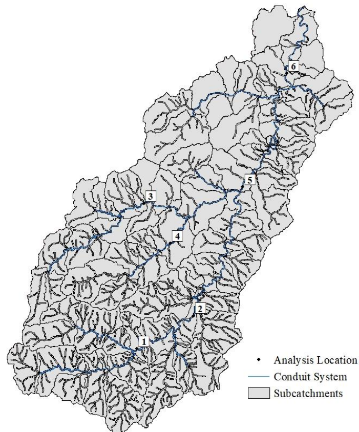
Figure 3.8. Scenario 1C required creation of a 150-foot buffer around the National Hydrography Dataset, which extends well beyond the conduit system shown in blue. For routing purposes, these buffers were made into their own subcatchments to allow for simulation of varying conditions in the buffer area.
