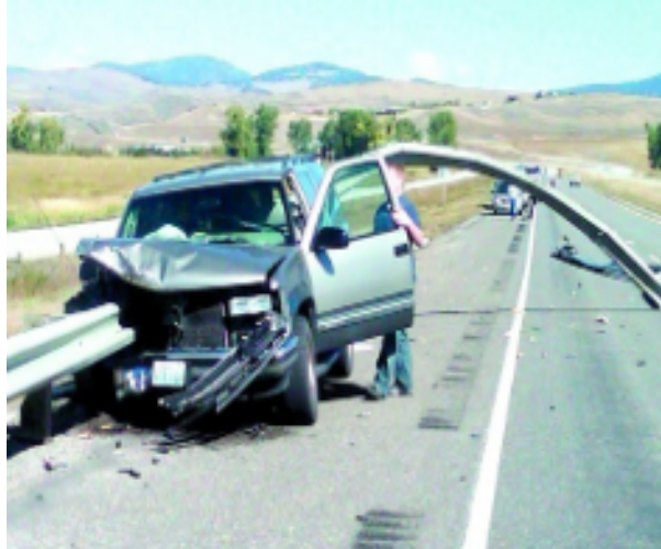
Figure 1.4: An Example of a Vehicle Crash with a Guardrail Blunt-End (Glennon & Engr., 2012)
