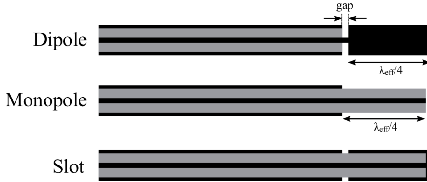
Figure 2-6: Original antennas: dipole, monopole, and slot (black metal, grey: dielectric).
