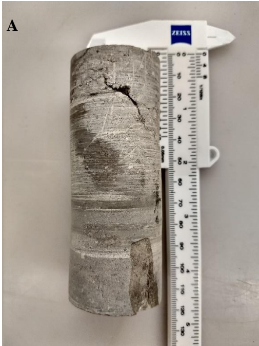
Figure 4-10: (A) 2891 ft cylindrical core sample, and (B) 2913 ft half cylinder core sample. Both core samples were obtained from the CO2-I #1 well. Note that these images were acquired after testing and that the fractures are a result of failure during the test.
