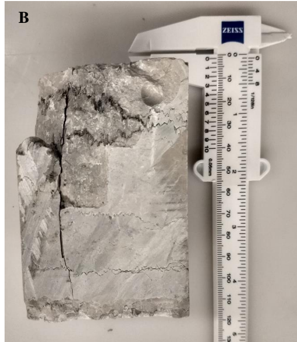
Figure 4-10: (A) 2891 ft cylindrical core sample, and (B) 2913 ft half cylinder core sample. Both core samples were obtained from the CO2-I #1 well. Note that these images were acquired after testing and that the fractures are a result of failure during the test.
