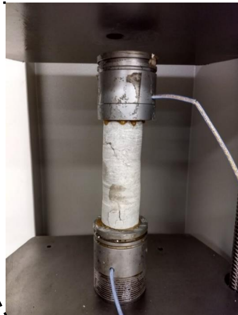
Figure 4-11: Core samples are placed in a hydraulic press between an ultrasonic transmitter and receiver. A thin film of honey is spread between the sample and the transmitter and receiver to ensure proper coupling. The transmitter and receiver are wired to a GCTS Testing Systems ULT-100 Ultrasonic interface, which is driven by the GCTS C.A.T.S. Ultrasonics software installed on the desktop computer located in Dr. Raef's lab.
