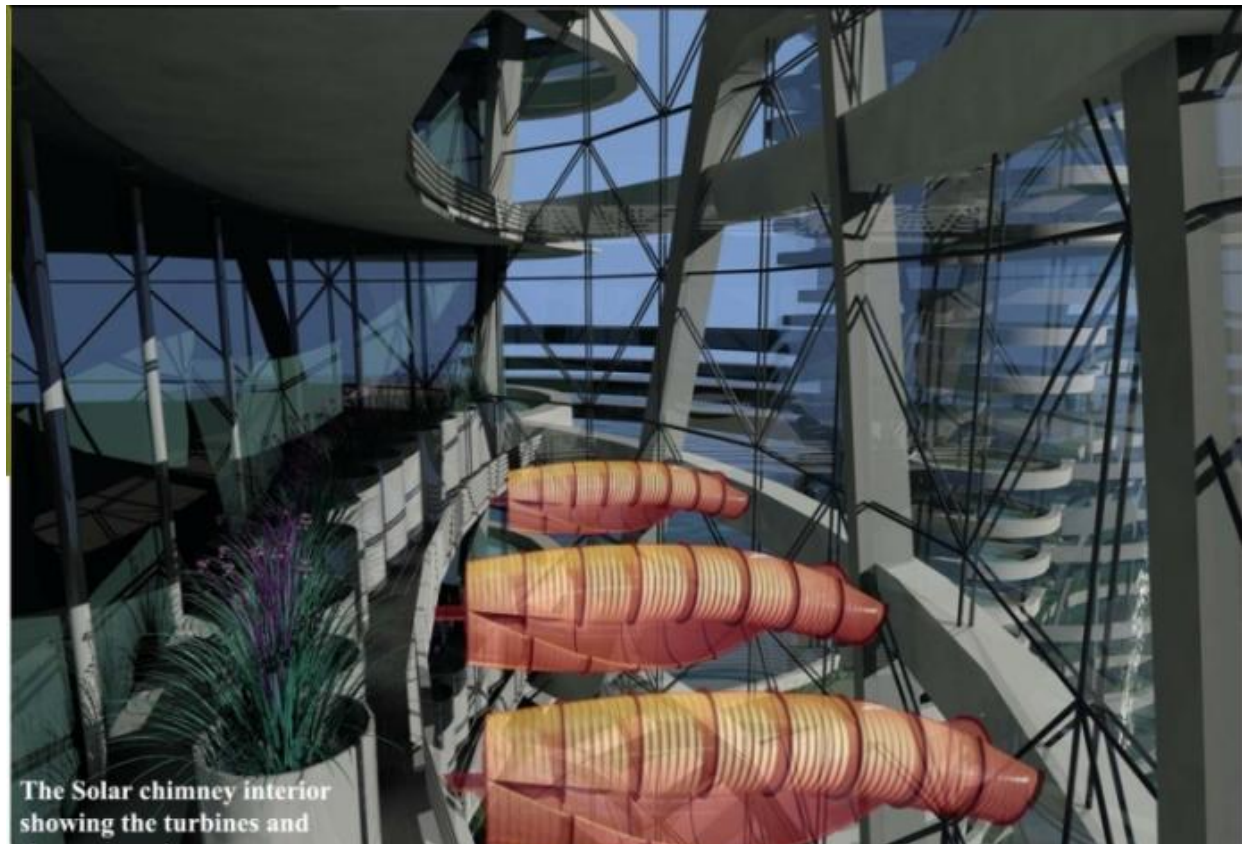
Figure 4.6 Interior view of the solar chimney showing the wind turbines (Design : Author)
