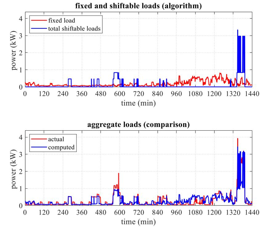
Figure 4.3: Disaggregated shiftable loads (top) and aggregate loads (bottom) for Day-1.
