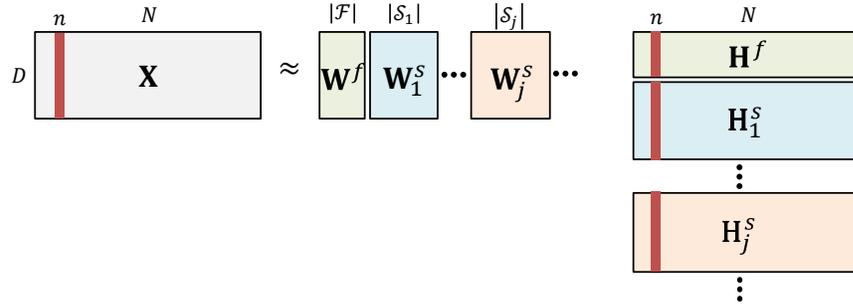
Figure 4.1: . Schematic of NMF factorization with separate basis and weight matrices for the fixed and shiftable loads.
