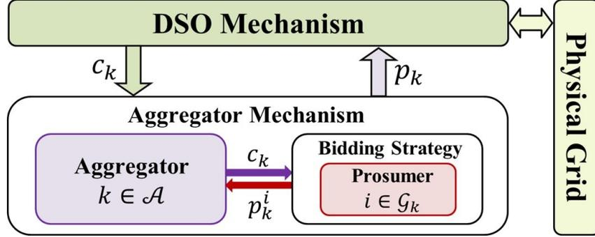
Figure 2.1: Schematic of the functional components of the grid and the bi-level flow of information between them.
