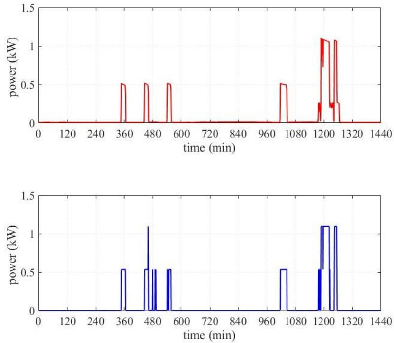
Figure 5.7: Shiftable load actual (top) and computed (bottom) for User-2.
