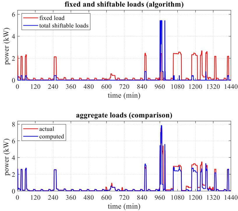
Figure 4.5: Disaggregated shiftable loads (top) and aggregate loads (bottom) for Day-2.
