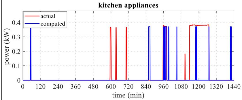
Figure 4.6: Disaggregated shiftable loads for Day-2.
