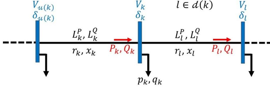
Figure 2.3: Distribution system radial branch model.
