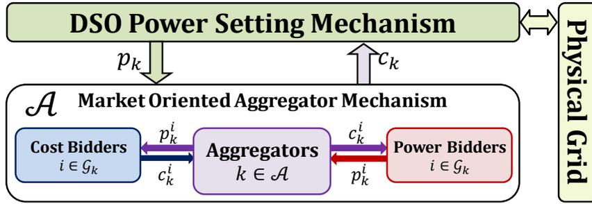
Figure 3.1: Schematic of market-driven bilevel mechanism
