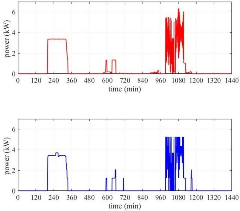
Figure 5.4: Shiftable load actual (top) and computed (bottom) for User-1
