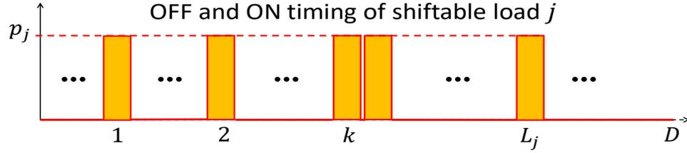
Figure 4.2: Illustrative usage profile of a shiftable load showing a maximum of  $L_j$  duty cycles, with each such cycle being a rectangular pulse of uniform peak  $p_j$ .
