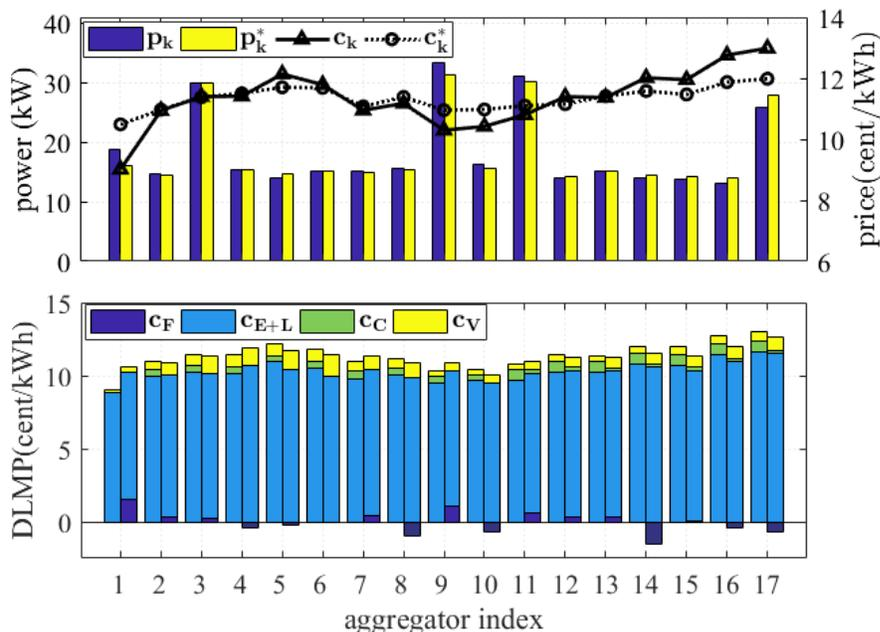
Figure 2.6: Results of Scenario-II showing unit costs and allocated power to each aggregator (top) and the DLMP components (bottom).
