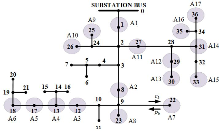
Figure 2.4: IEEE 37 bus system with aggregators indexed A1 – A17.
