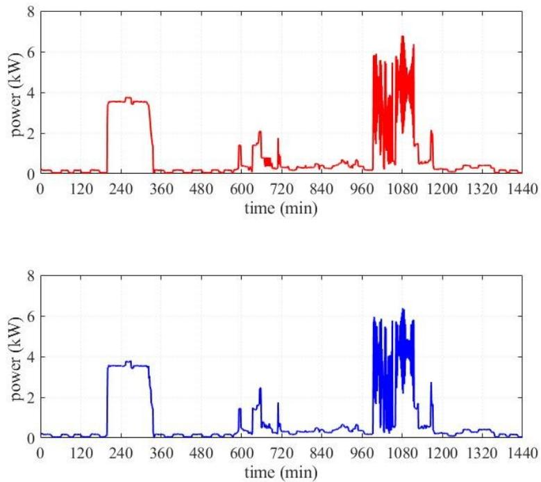
Figure 5.6: Aggregate load actual (top) and computed (bottom) for User-1.
