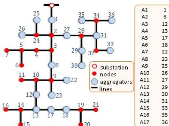
Figure 3.6: IEEE 37-bus system used as simulation platform
