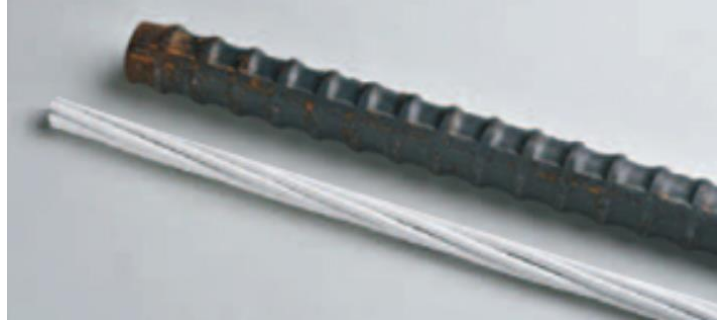
Figure 4.1-3: Size Comparison of Strand Rods vs. #4 Rebar. Reprinted from 'CABKOMA' by Komatsu Matere
