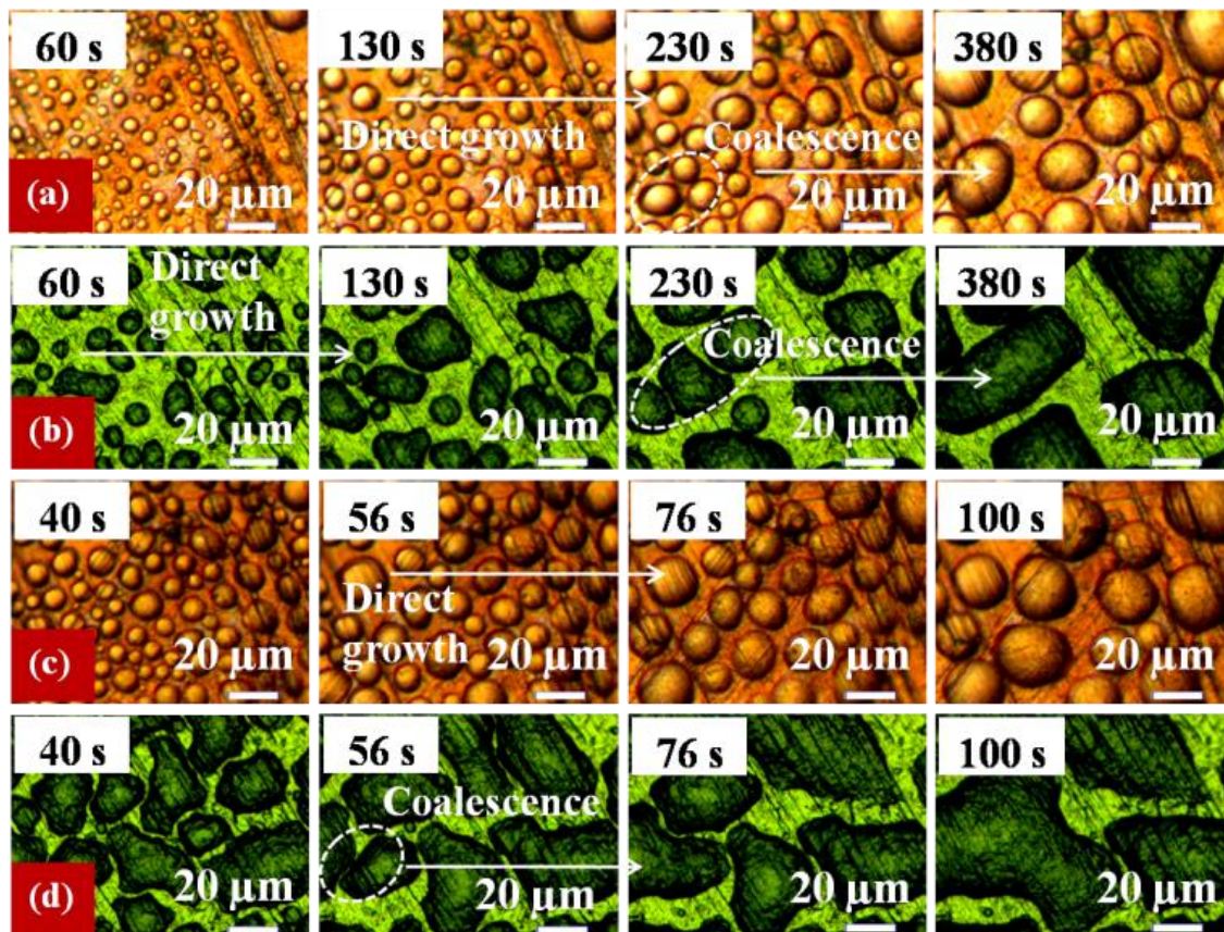
Figure 6.3 Droplet growth mechanism for (a) plain copper, 40% RH (b) GO coated copper, 40% RH (c) plain copper, 60% RH and (d) GO coated copper, 60% RH [110].
