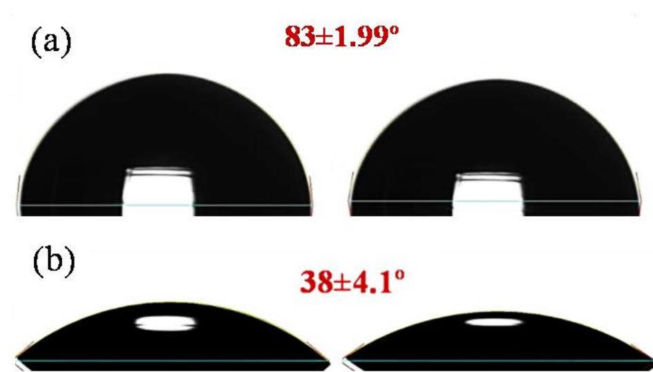
Figure 3.3 Apparent average contact angle measurement for the injected water droplet on (a) nanopillar surface (b) silicon surface [82].
