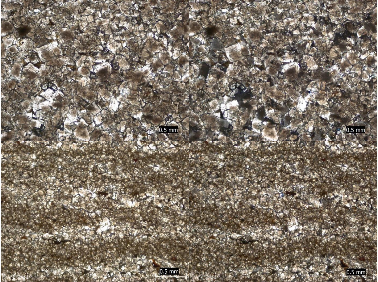
Figure B.44: Thin section photomicrographs of Muddy dolostone at 5841.83' from the Rich C #7 well. From left to right, the photomicrographs are in PPL, XPL (same microscope location as previous image), PPL, and XPL (same microscope location as previous image).
