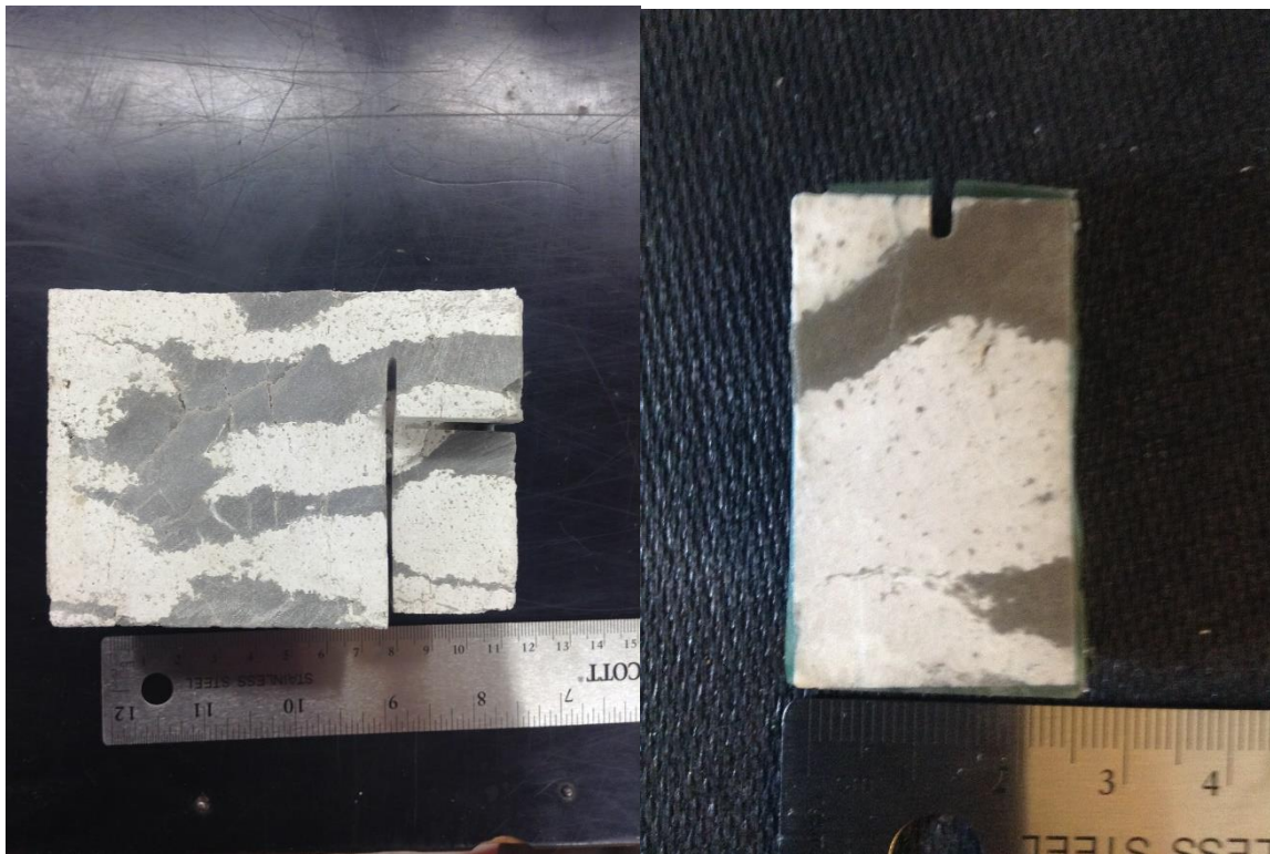
Figure B.15: Cored section of Cherty dolomite in the Viola Ls. from Rich C #7 (left) and thin section plug of this core piece taken at 5822' (right).
