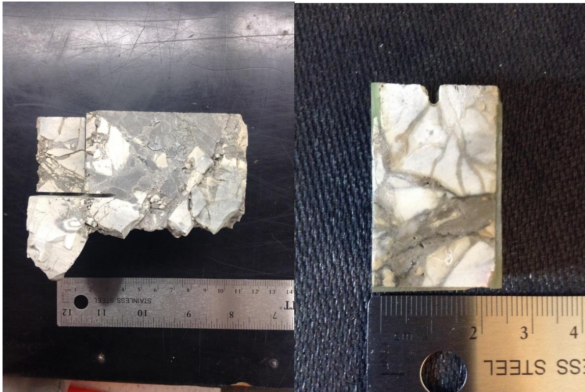
Figure B.6: Cored section of Intraclastic breccia in the Viola Ls. from Rich C #7 (left) and thin section pluf of this core piece taken at 5811.66'(right).
