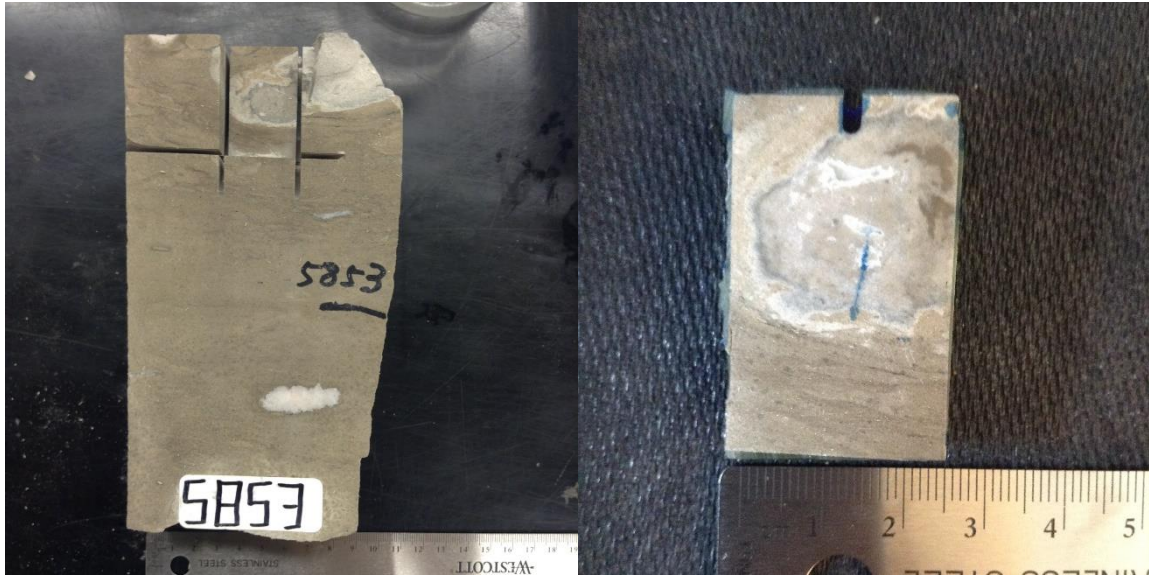
Figure B.48: Cored section of Muddy dolostone in the Viola Ls. from Rich C #7 (left) and thin section plug of this core piece taken at 5852.66'(right).
