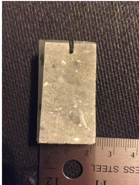
Figure B.2: Cored section of Intraclastic rudstone in the Viola Ls. from Rich C #7 (left) and thin section plug of this core piece taken at 5808'(right).
