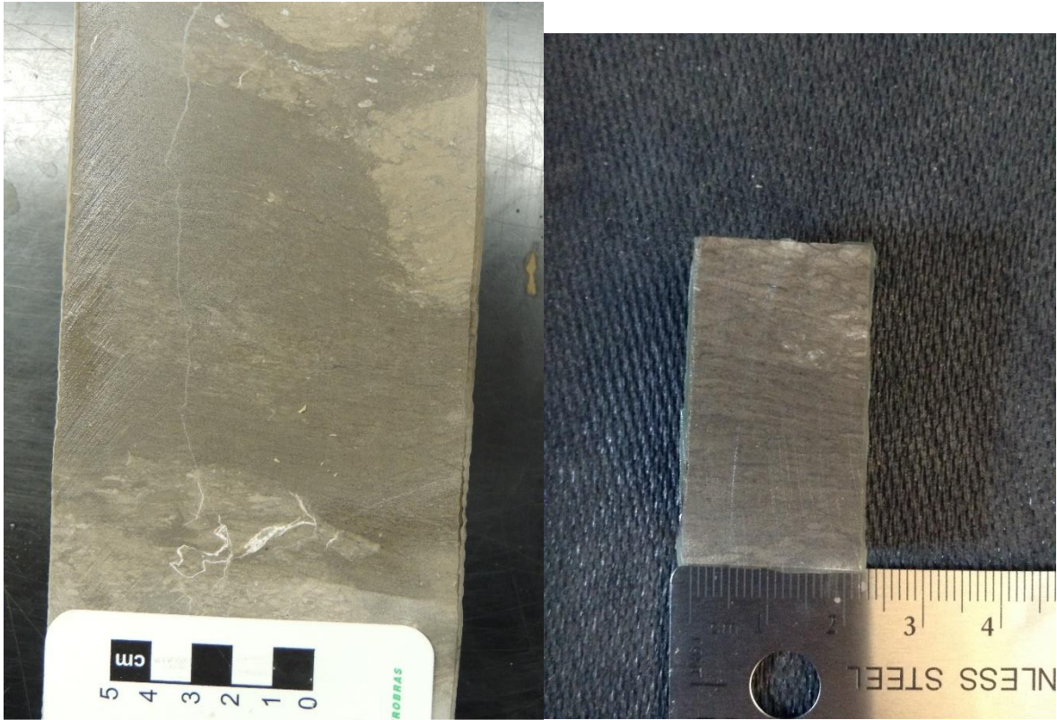
Figure B.67: Cored section of Muddy dolostone in the Viola Ls. from Rich C #7 (left) and thin section plugs of this core piece taken at 5865.5'(right).
