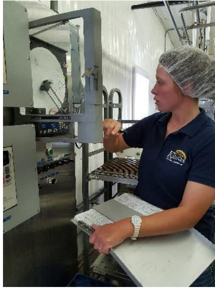
Figure 3.8 An inspector examining the real-time temperature recorder accuracy of the pasteurization system.
