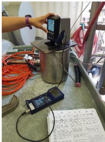
Figure 3.7 The temperature alarm probe testing with the KDA-calibrated thermometer.
