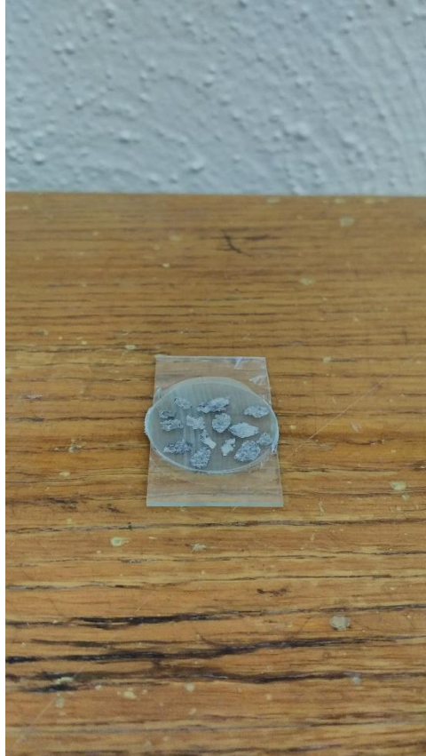
Figure 11: Images in order from top to bottom and left to right. Image of cutting blanks inside of pill cups and labelled by well name, depth, and circulation time. Image of cutting blank with the pill cup removed and the top side, the side with no cuttings, being flattened using sandpaper, preparing it to be placed on the Hilquist grinder. Image of blank placed
