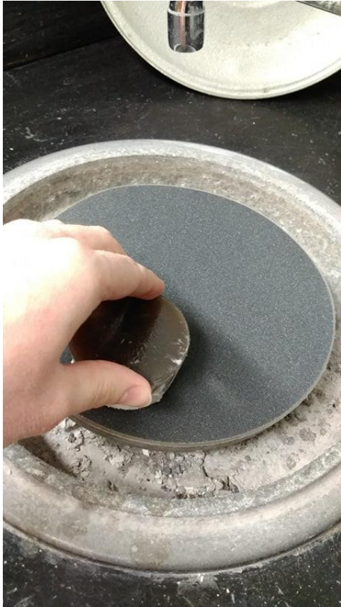
Figure 12: Images in order from top to bottom and left to right. Image of a thin section mounted in the thin section holder. Image of the table top disk sander and the sand paper that is applied to the surface of the sander. Image of the sand paper after it had been applied to the disk sander. Image showing the faucet that was used to apply a thin layer of water onto the sand paper. Image showing the method that thin sections were held in place on the disk sander using the thin section holder. Image of the speed controller, speed was always set to I.
