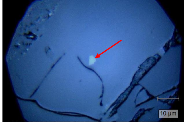
Figure 21: A reflected light imaged captured by the Renishaw InVia Raman Microscope showing a representative target mineral from analysis 5-1. The target is the yellowish crystal near the center of the image indicated by the red arrow.
