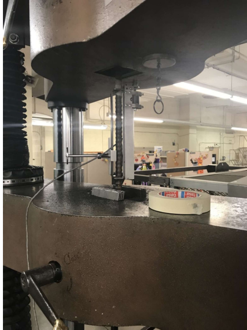
Figure 6-4 Steel tensile test
