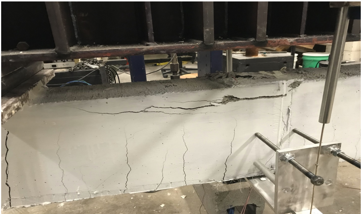
Figure 6-18 Tested beam concrete failure
