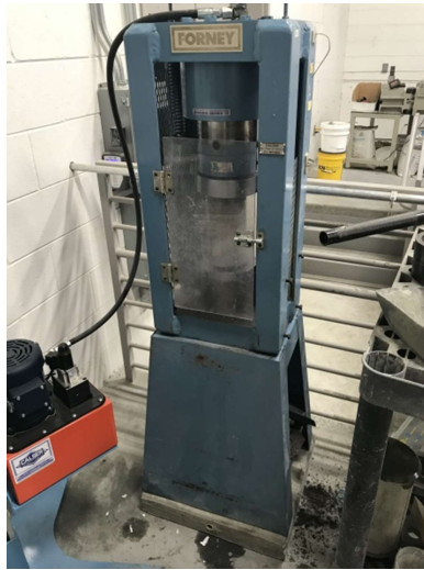
Figure 6-2 Concrete cylinder compression test (before test)
