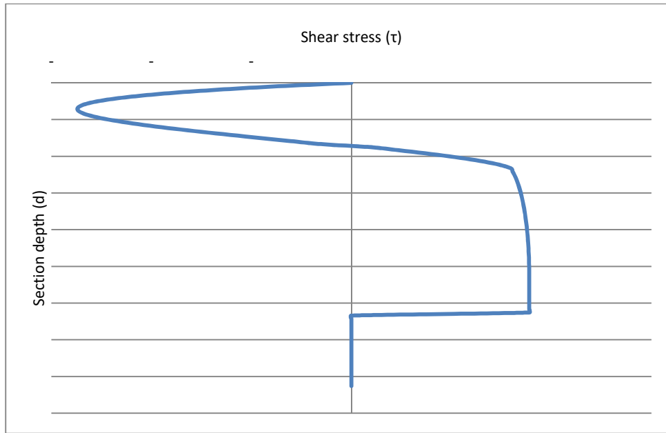
Figure 3-11 Typical post yielding shear stress distribution
