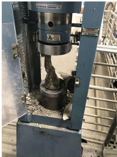
Figure 6-3 Concrete cylinder compression test (after test)
