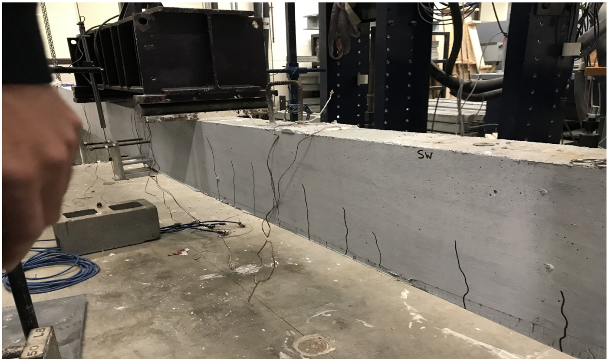
Figure 6-20 Tested beam principal tensile cracking (side two)
