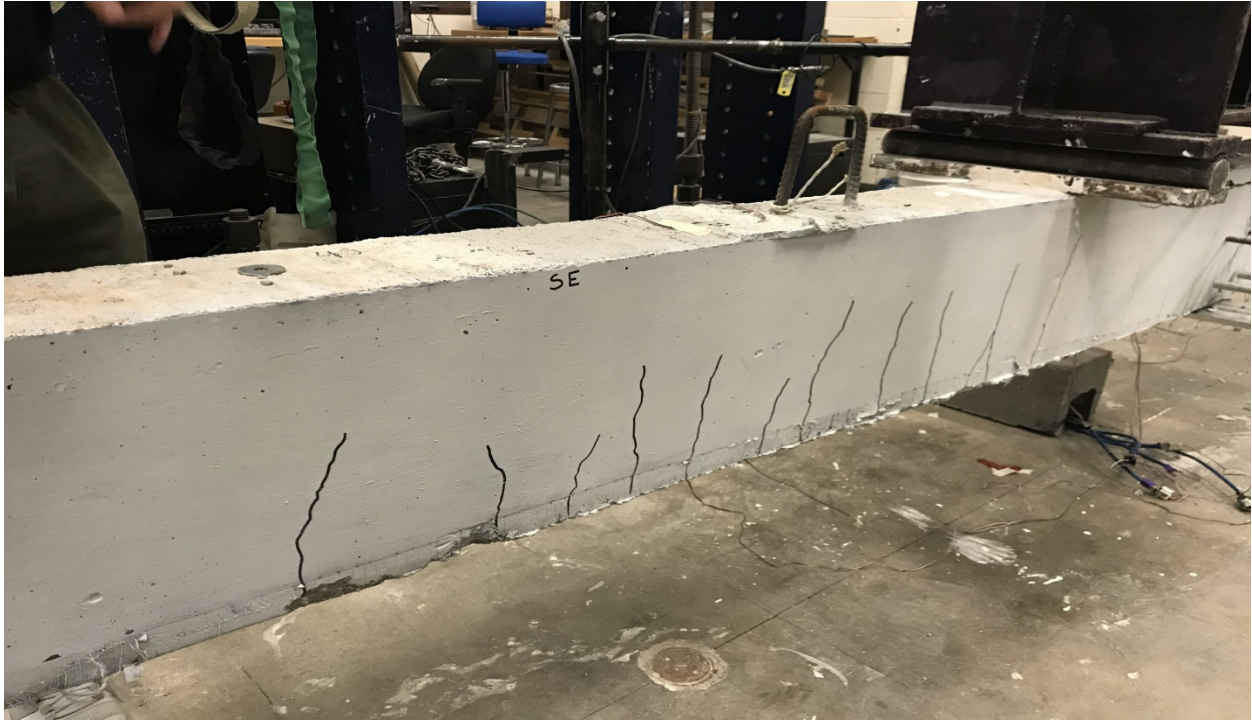
Figure 6-19 Tested beam principal tensile cracking (side one)
