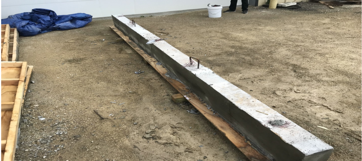
Figure 6-14 Casted reinforced concrete beam
