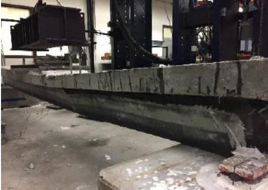
Figure 5-19 Beam T3 after the failure
