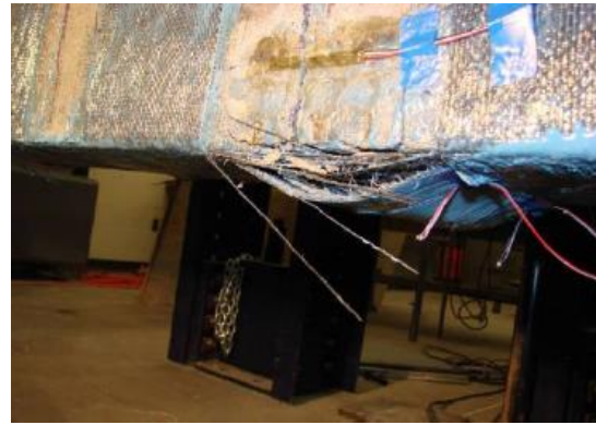
Figure 5-29 Beam R5 after the failure
