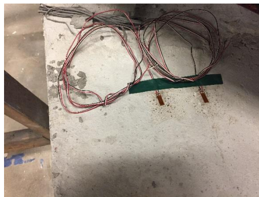
Figure B-2: After soldering the leadwires on a T beam surface
