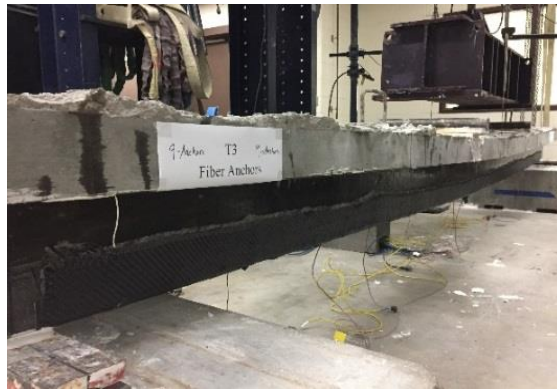
Figure 6-25 Beam T3 after the failure
