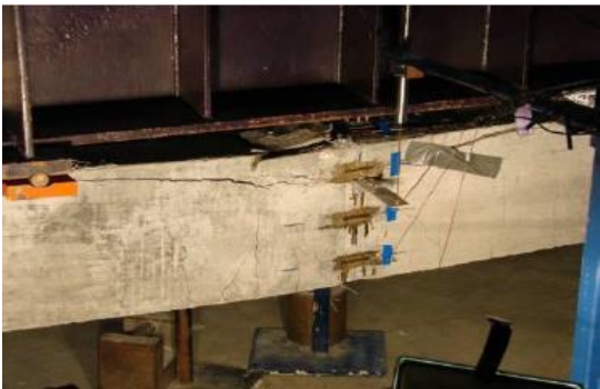
Figure 7-14 Control beam CBR after the test
