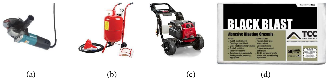
Figure 4-7 Tools and materials used for roughening the surface (a) a grinder; (b) sandblaster; (c) pressure washer; abrasive blasting sand
