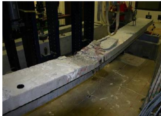
Figure 6-15 Control beam T1 after the test
