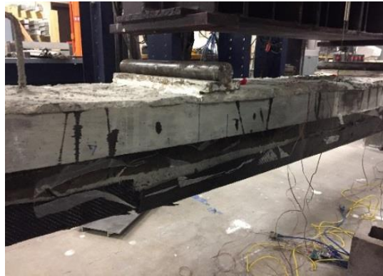
Figure 6-18 Failure of the beam T2
