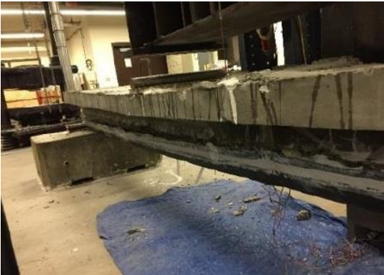
Figure 5-12 Beam T2 after the failure
