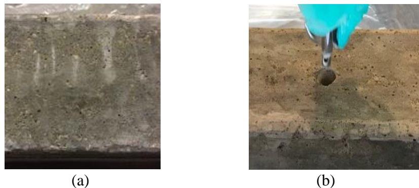
Figure 7-3 Surface preparation for the beams (a) roughening the surface; (b) drilling and cleaning the predrilled holes
