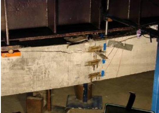
Figure 5-24 Control beam R1 after the test
