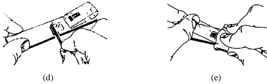
Figure B-1: Installation of the strain gauges (a); applying a piece of PCT-2M tape (b); position the gage into the place (c); letting up the tape (d); applying the adhesive and (e) laying down gage onto the adhesive.
