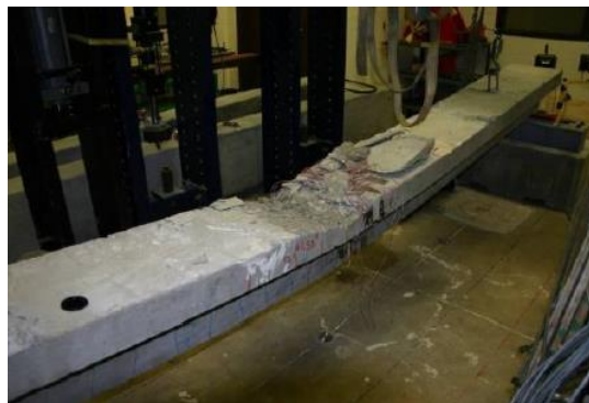
Figure 5-9 Control beam T1 after the test
