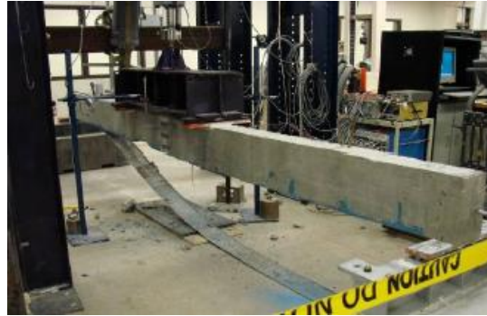
Figure 7-18 Beam R2 after the failure
