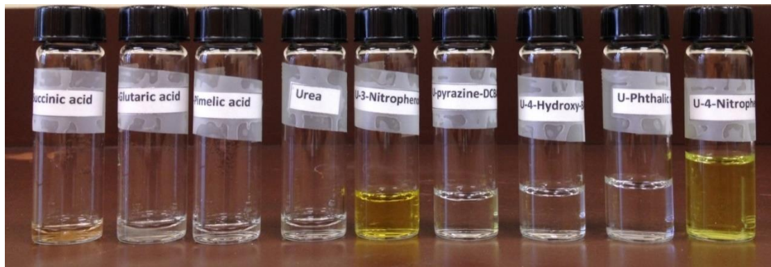
Figure 9.11 Qualitative analysis of urea and urea-co-former co-crystals in distilled water
