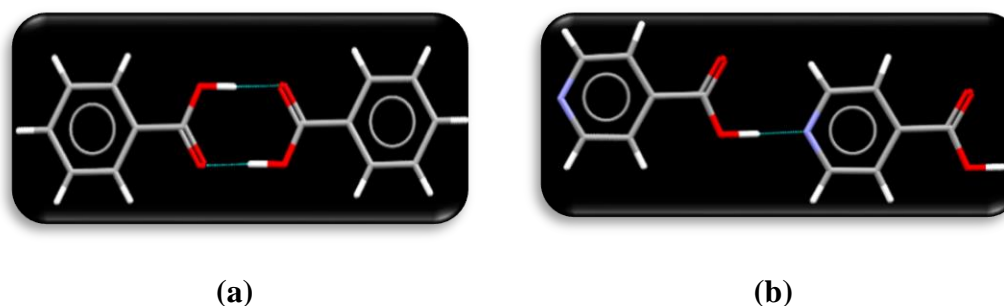
Figure A.16 Hydrogen-bonding synthon observed in the crystal structure of (a) benzoic acid and (b) isonicotinic acid.
