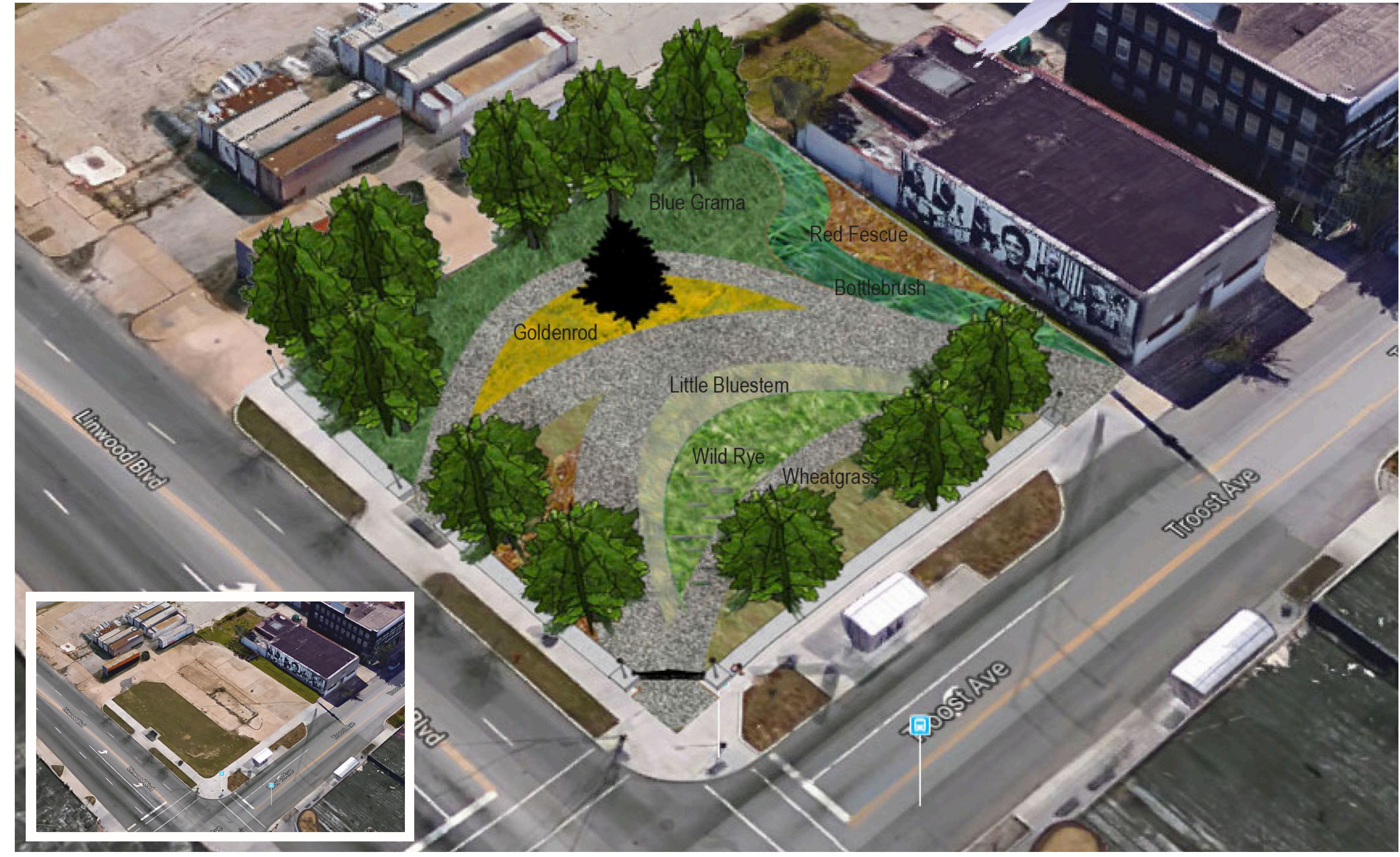
Figure 19. The empty lot would be transformed into a demonstration neighborhood park, using phytotechnology for site remediation. The plants will slowly remove contaminants from the soil.
