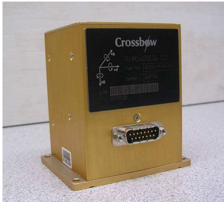
Figure 3.7 The AHRS400 Gyroscope with its Coordinate System Illustrated on the Front Face
