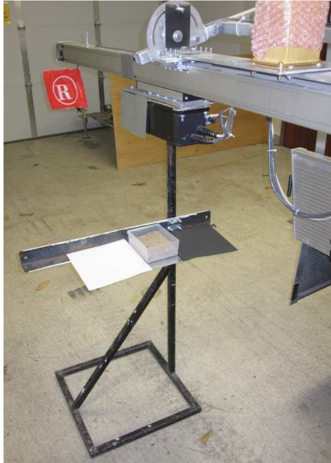
Figure 4.2 The Platform for the Laser Scanner and the Targets
