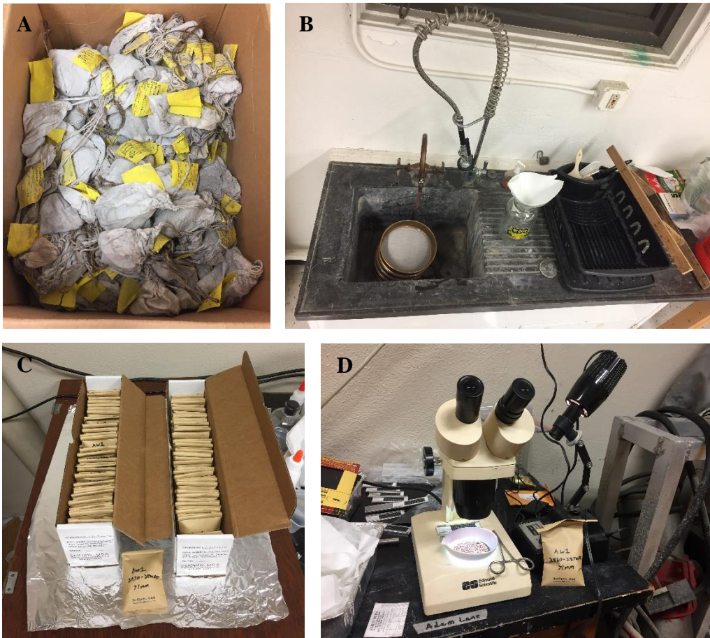
Figure 24: The drill cutting cleaning and sorting process. (A) Unprocessed drill cuttings. (B) Area of washing and wet sieving. (C) Sorted and packed drill cuttings. (D) Stereo microscope used for examination.
