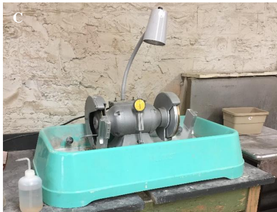
Figure 26: The thin section production process. (A) Drill cuttings in ice cube trays ready to be immersed in resin. (B) Drill cutting plugs drying in a fume hood after attachment to frosted slide. (C) The Hillquist thin section machine used for frosting slides, sawing, and grinding. (D) The finished thin sections ready for examination.
