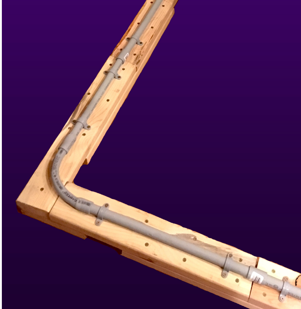
Figure 3-10: Factory Elbow Experiment Construction
