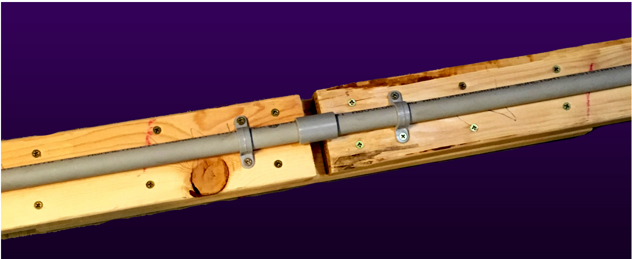
Figure 3-8: Midpoint Connection in Place of Elbow Entity
