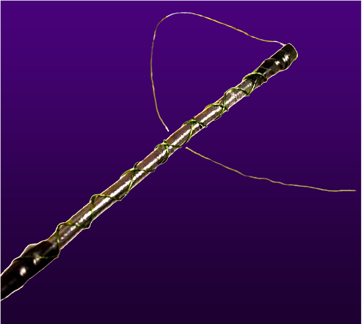
Figure 3-5: Applied Conductor Header Midway Through Construction
