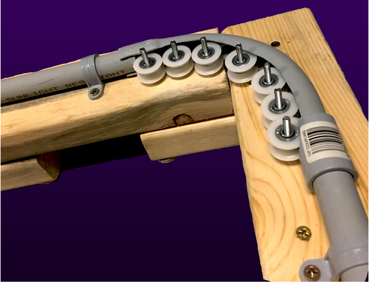
Figure 1-1: Modeled Product Experiment Construction Prior to Securing Roller Elevations
