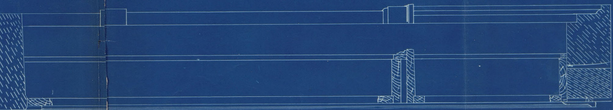
SECTION THROUGH FRONT DOOR SCALE 3/4"=1'
