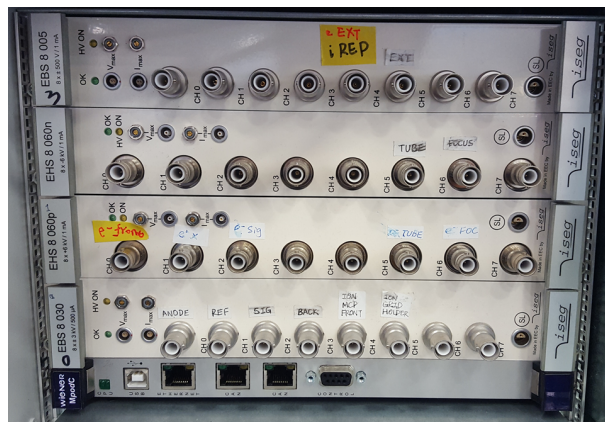
Figure C.1: Picture of the universal power supply system used in the double-sided VMI experiments.
