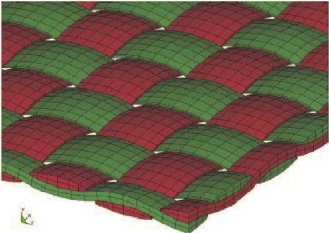
Figure 2-6: Yarn level FE model [22]
