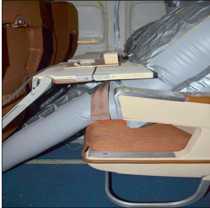
Figure 4.3 Sampling Ports Used for Testing at Breathing Level of Seated Infant Passengers
