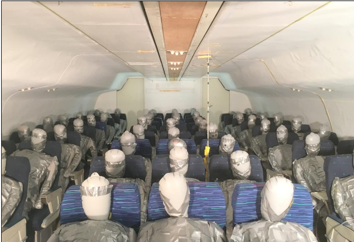
Figure 3.17 Thermal Manikins Occupying All Seats Inside the Boeing 767 Mockup Cabin
