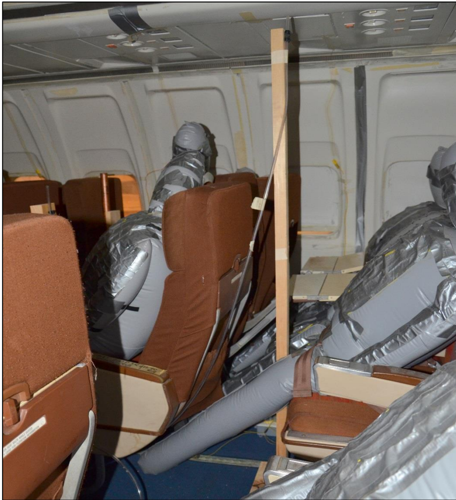
Figure 4.5 Sampling Ports Used for Testing at Breathing Level of Standing Passengers
