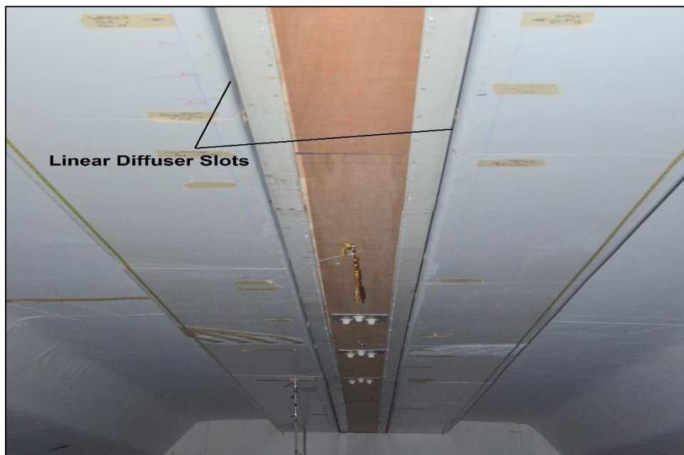
Figure 3.6 Linear Diffuser Slots Inside the Boeing 767 Cabin
