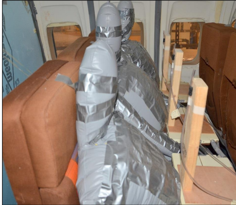
Figure 4.2 Sampling Ports Used for Testing at Breathing Level of Seated Adult Passengers
