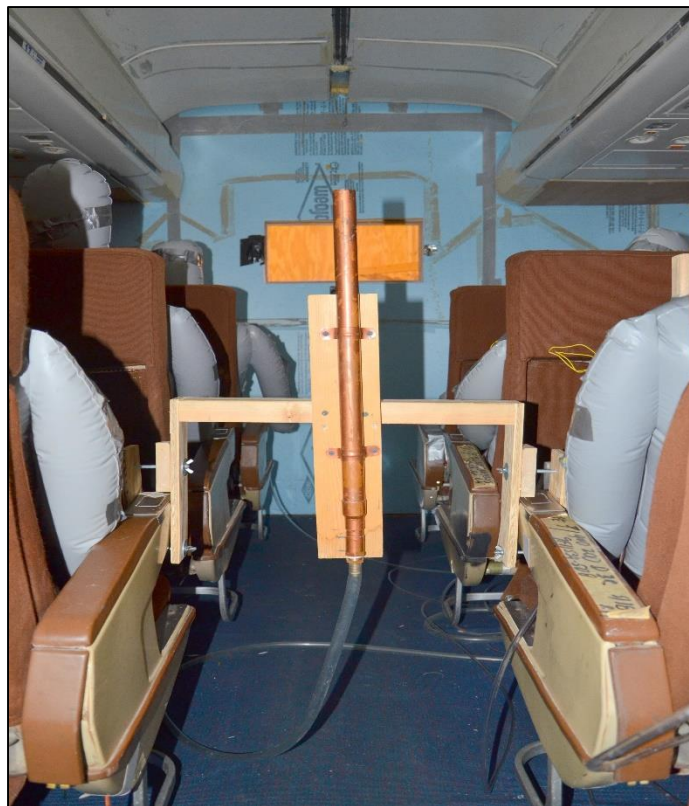
Figure 4.10 Tracer Gas Injection Apparatus for Tracer Gas Dispersion Study
