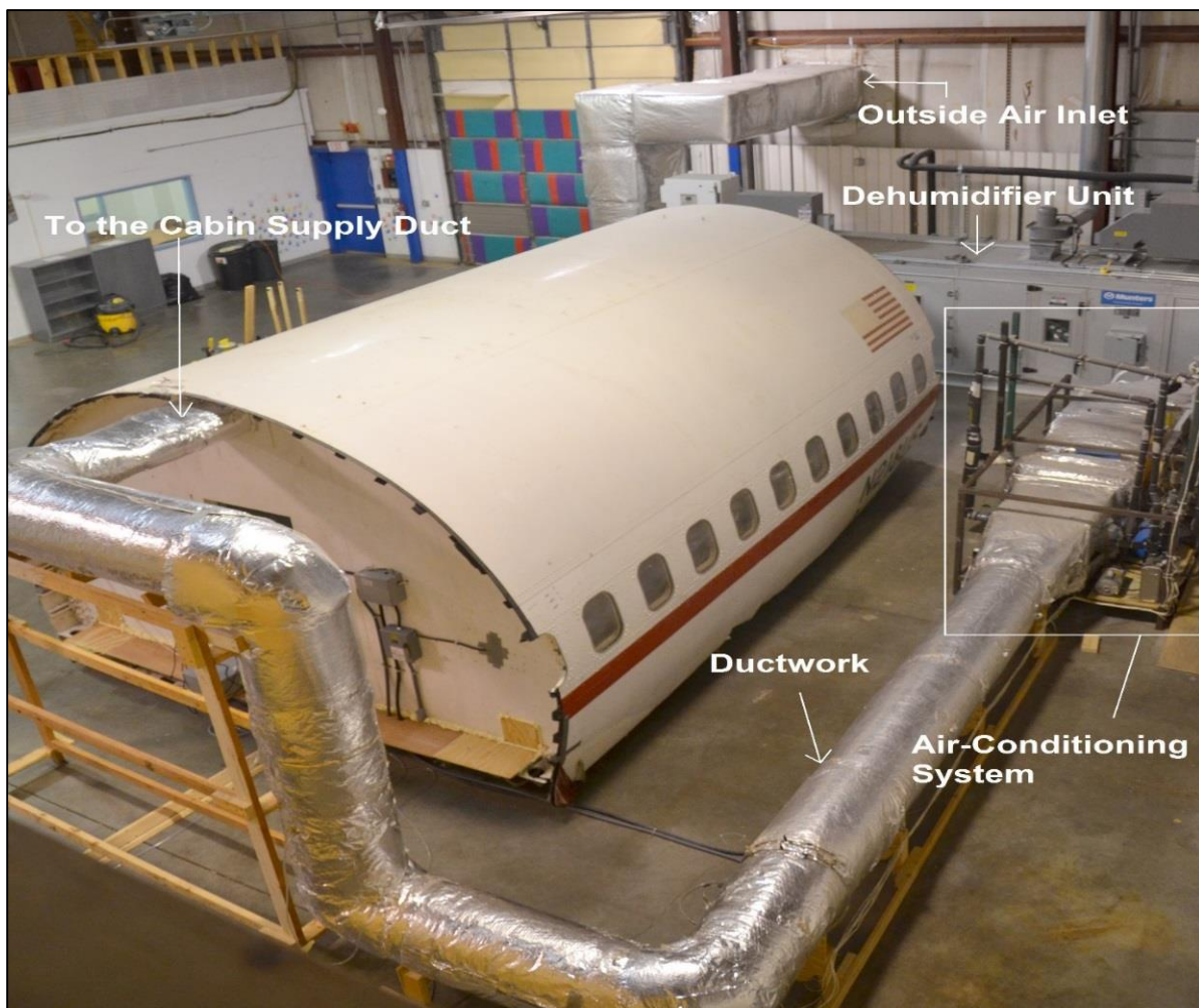
Figure 3.18 Ductwork for the Boeing 737 Mockup Cabin
