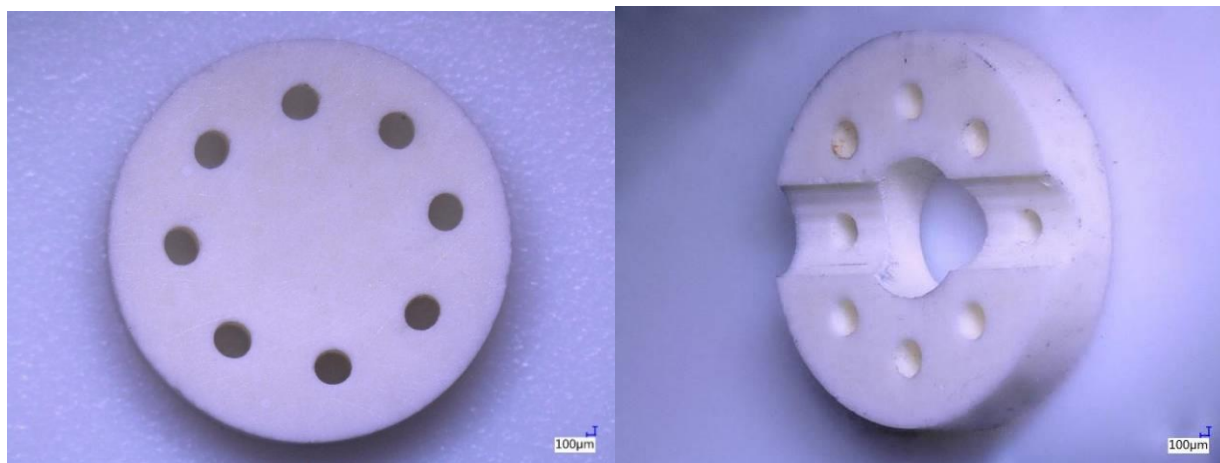
Fig. 6.7 Each MPFD node was composed of two disks (left) and 2 spacers (right) creating the ionization chamber with a channel exposing the appropriate anode and cathode wires.
