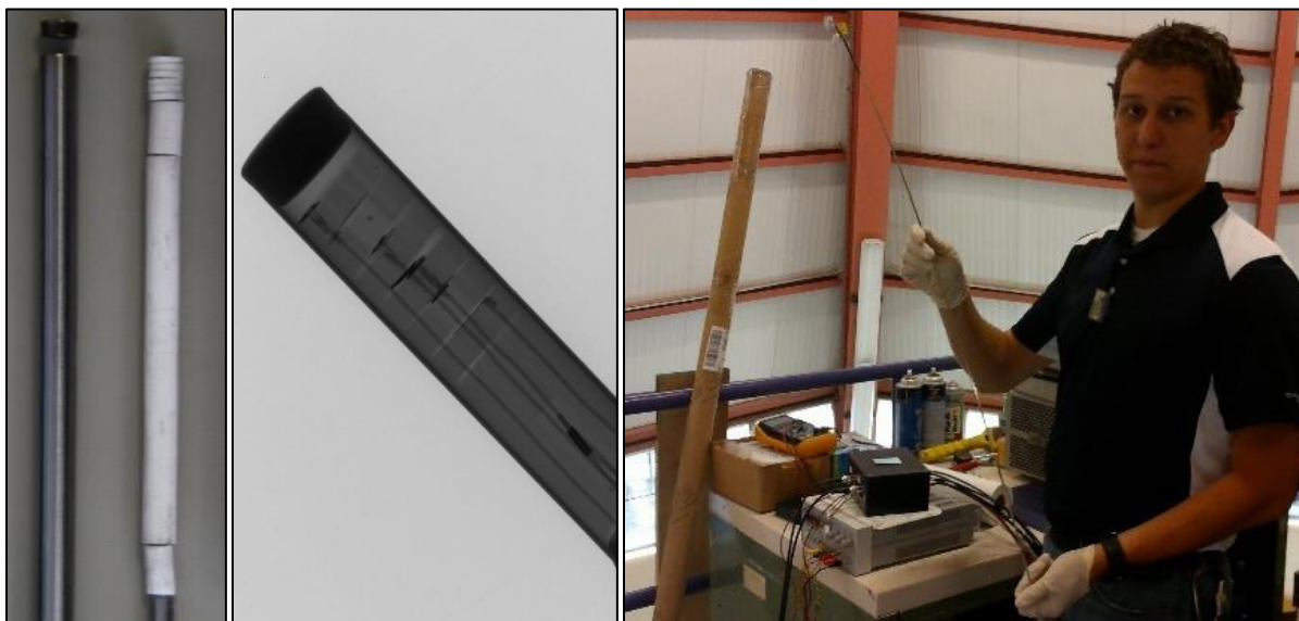
Fig. 5.7 The first encapsulated MPFD utilized a parallel plate geometry with conductive adhesive and was assembled on the end of several feet of custom mineral insulated cable.
