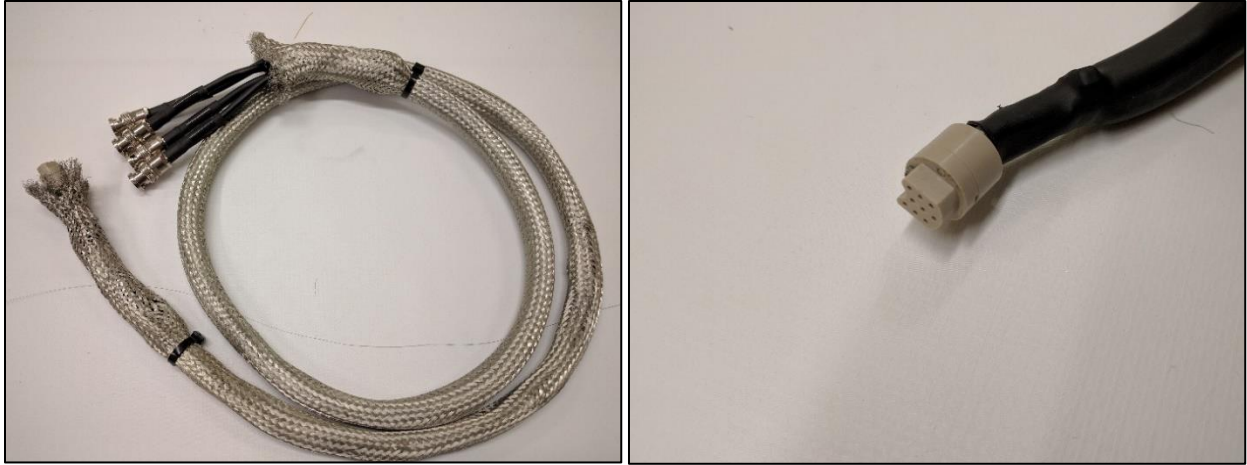
Fig. 5.17 An electronic feedthrough (MDC 1039601) and electronic feedthrough plug (MDC 1150101) connected the MPFD array anode and cathode wires with the signal cables.
