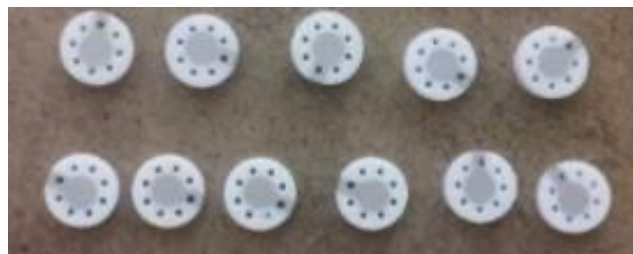
Fig. 4.16 Specialized evaporation masks were used to index the contact pad with 1 hole in the alumina.
