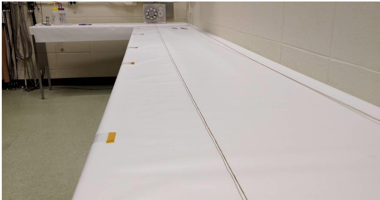
Fig. 6.36 Braiding the anodes around the cathode wire adds rigidity to the array while still allowing the array to bend as necessary.
