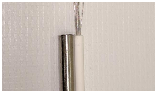
Fig. 6.14 The silica insulation was used throughout the length of the stainless-steel encapsulation tube. Fiberglass insulation (not pictured) was used to insulate the remaining 4 inches of wire which was connected to the electrical plug.
