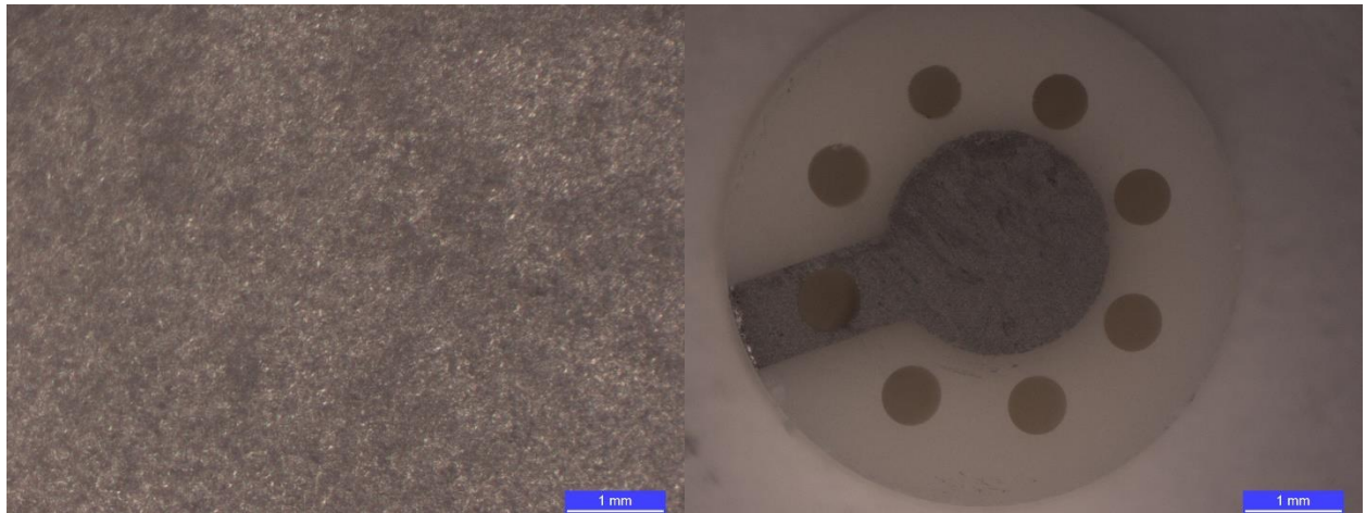
Fig. 4.8 Thin evaporated layers, in conjunction with a thin adhesion layer (Ti/Pt 50Å/500Å respectively) produced uniform coatings on the alumina substrates.
