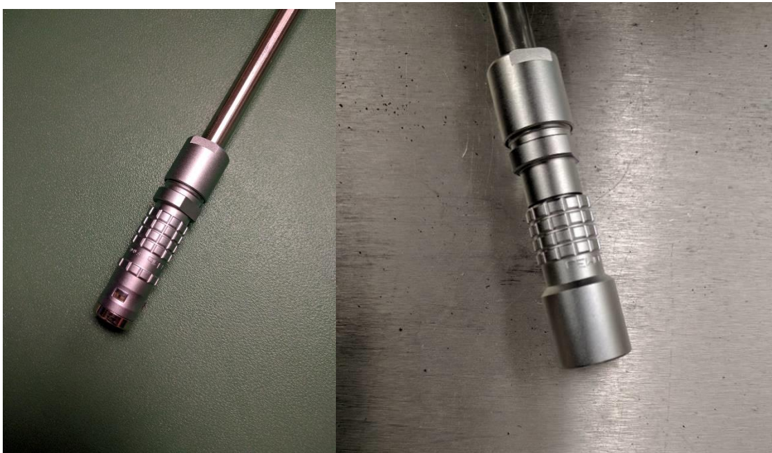
Fig. 5.19 The modular MPFD array utilized a Lemo (FG.1K.308.CLAK80, left) plug on the array with a Lemo (PHG.1K.308.CLLK75, right) receptacle on the multi-pair shielded cable.
