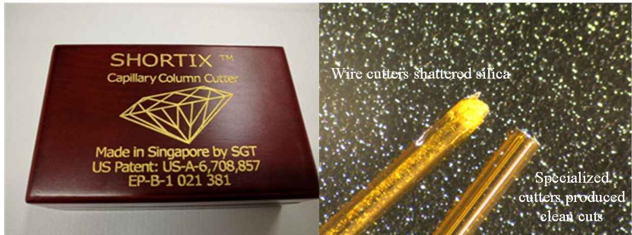
Fig. 5.13 The use of a specialized capillary tube cutter improved the quality of the assembled MPFD array, reducing fracturing and improving wire coverage [34].
