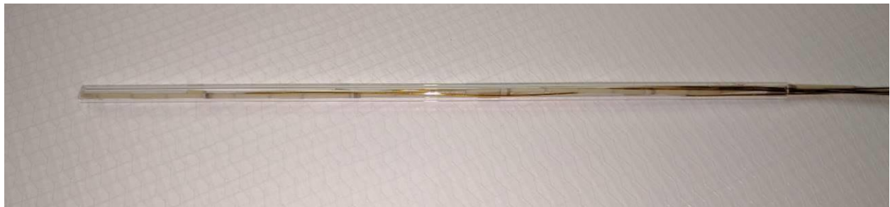
Fig. 6.37 A small quartz tube was added to the MPFD region of the array to reduce the likelihood of shorting between the anode terminations and the flux port wall.
