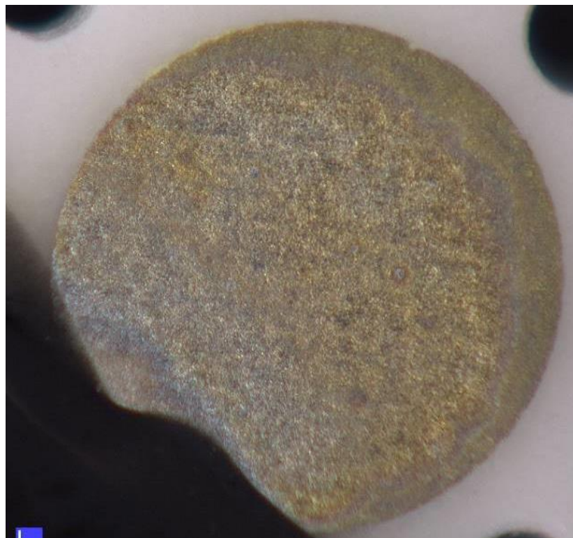
Fig. 4.31 Determining the optimal voltage-sweep interval improved the quality of the electrodeposited layer, shown on sample A12.g.
