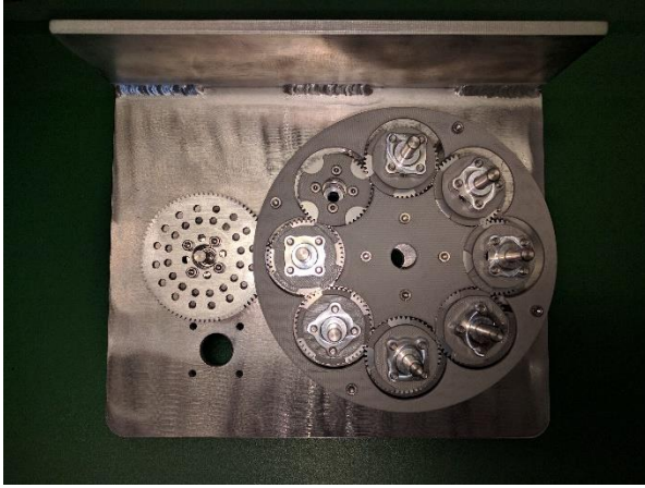
Fig. 5.15 Although braiding by hand was sufficient for 2-node MPFD arrays, expansion to 5-nodes called for a mechanical braider to be developed.
