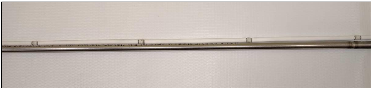
Fig. 6.11 Four MPFD nodes were constructed with 10.48-cm (4 1/8-in.) silica spacers between each node. The total distance between the node center points was 11.11-cm (4 3/8-in.) due to the length of each MPFD node.
