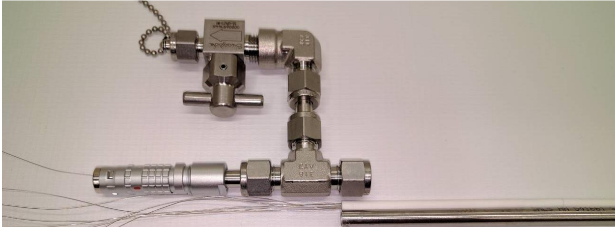
Fig. 6.15 The vacuum/fill assembly was mounted next to the electronic plug to allow the anode and cathode wires to pass out of the encapsulation tube through the electronics plug.
