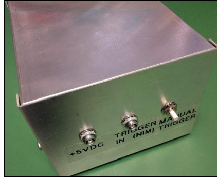
Fig. 5.29 The MPFD emulator box was be used in place of a full-scale MPFD array for bench-top electronics testing and optimization.
