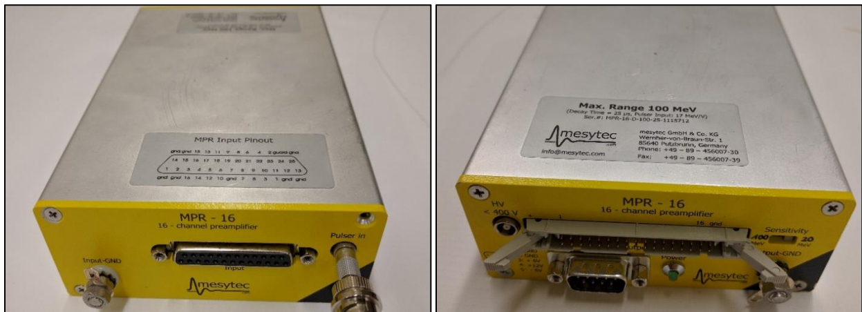
Fig. 5.27 The MPR-16_V100 preamplifier supports 16 channels of operation with a differential output signal which couples to a differential-mode MSCF-16 [40].
