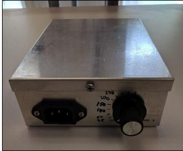
Fig. 5.22 Lithium-foil neutron detectors used a custom-built electronics system which included high-voltage supply, preamplifier, shaping amplifier, and a preset discriminator [37].
