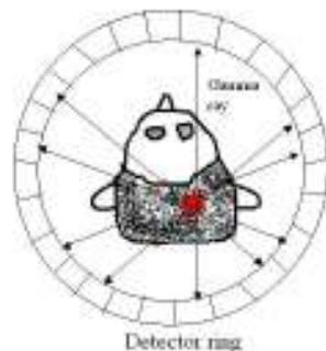
Data acquisition with a PET machine is the final step in the process. PET detectors arranged in a ring collect the signals coming out from the patient body as shown in Figure 2.1. The processing of data extracts information related to the tracer's activity in the body. Finally interpretation of results is produced in the form of scan, which is analyzed to diagnose the illness or abnormality of a tissue.
