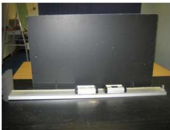
A large board is placed as a barrier in front of the track such that a student sitting behind the barrier can see the carts only when they reach the end of the track but not the location at which carts were released (Figure 4.1). Another student sitting on the other side of this board
