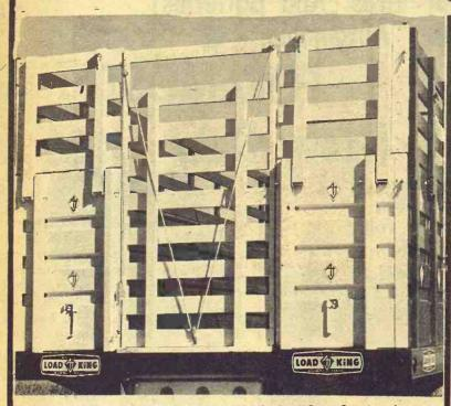
The Load King specially designed understructure has built-in clearance frame for hoist, eliminating the need to cut across members. The platform has a heavy duty reinforced framed opening for convenient hoist mounting. Flooring fastened from underneath; no bolt heads to protrude, no depressions to cause splintering and rotting. Get the truck bed that's built by Kansans, distributed by Kansans — Used by Everyone.
