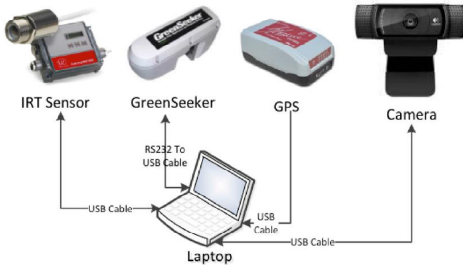
Figure 3.1 Integrated hardware components of Phenocorn.
