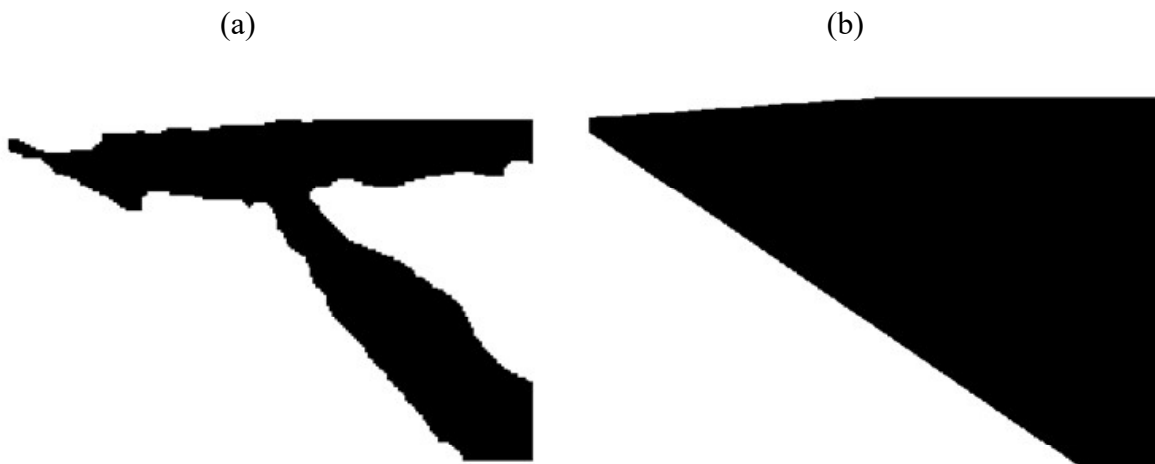
Figure 5.26 Pixel groups with concave shapes (a) and convex hull of a concave shaped pixel group (b).
