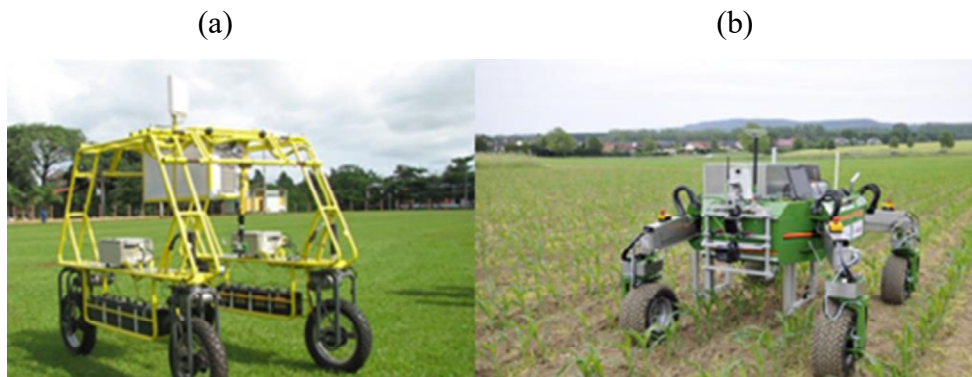
Figure 4.4 Two types of adjustable robot chassis for phenotyping (Rubens et al., 2011; Biber et al., 2012).
