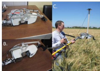
Figure 3.3 A and B. Custom mounting bracket to hold individual sensors. C. Using the Phenocorn as a handheld platform in the field, Ciudad Obregon, Mexico (Crain et al., 2016).
