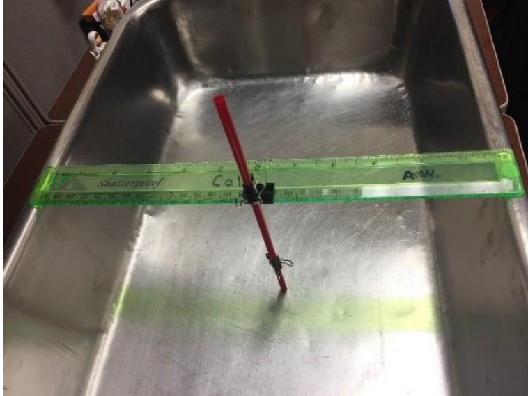
Figure F-4: Ruler and Binder Clip System Implemented to Stabilize Data Logger Probe in the Center of the Pan and Food Product
