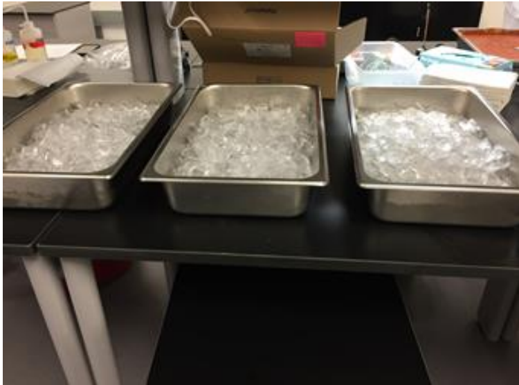
Figure F-6: Examples of Cover and Cooling Treatments Applied to Pans
