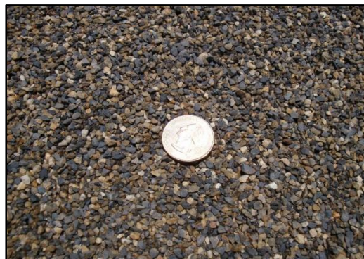
Figure 3.3 Chinese calcined bauxite aggregate used in this study
