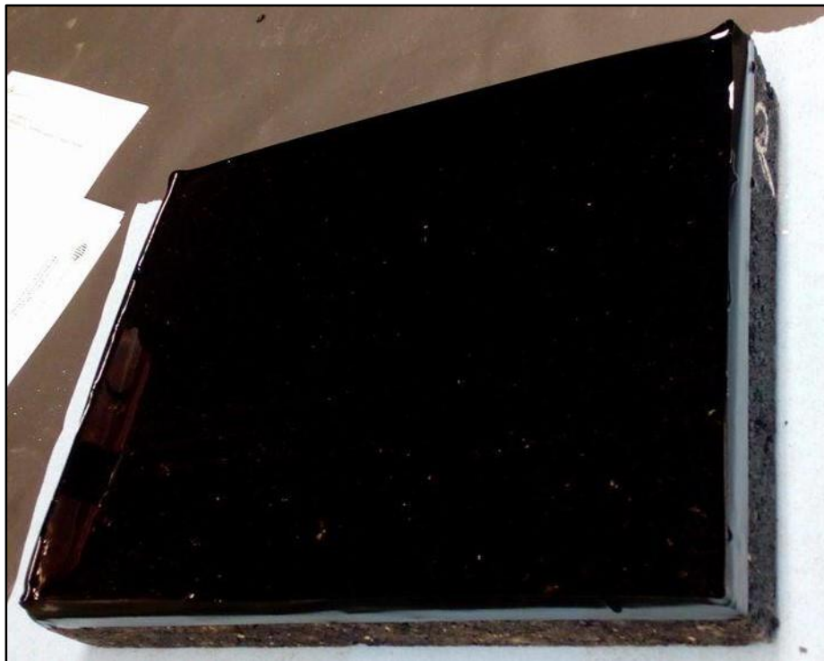
Figure 3.15 Slab covered with epoxy
