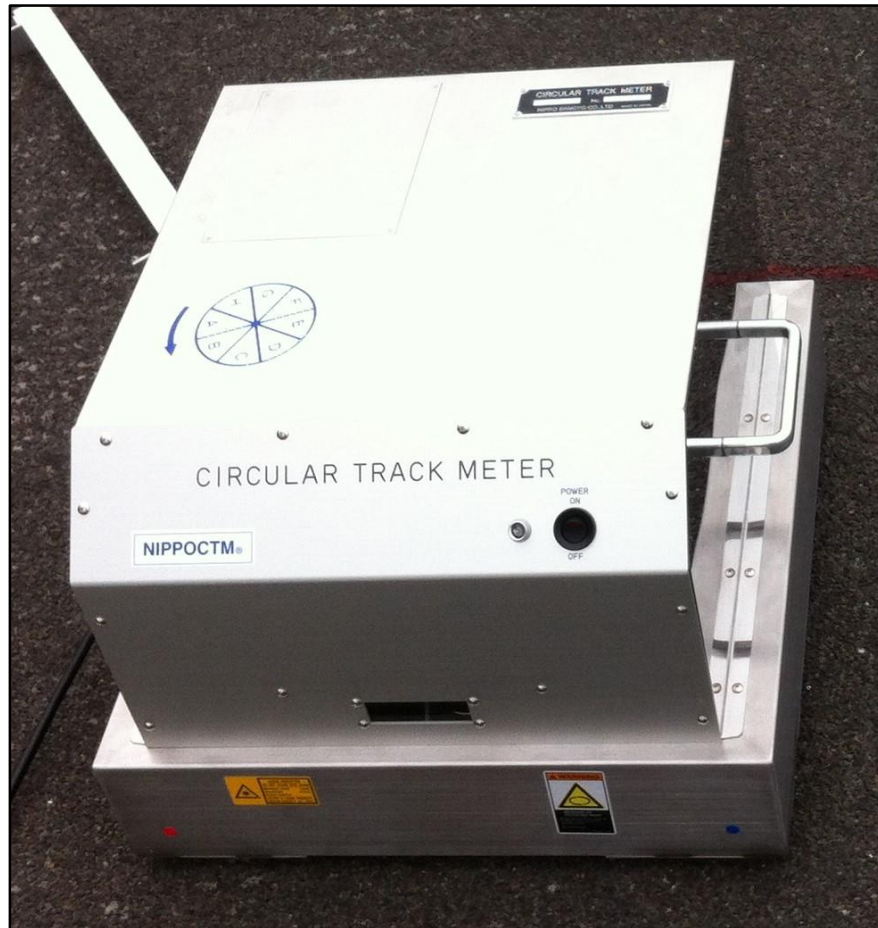
Figure 3.17 Circular track meter for measuring texture depth
