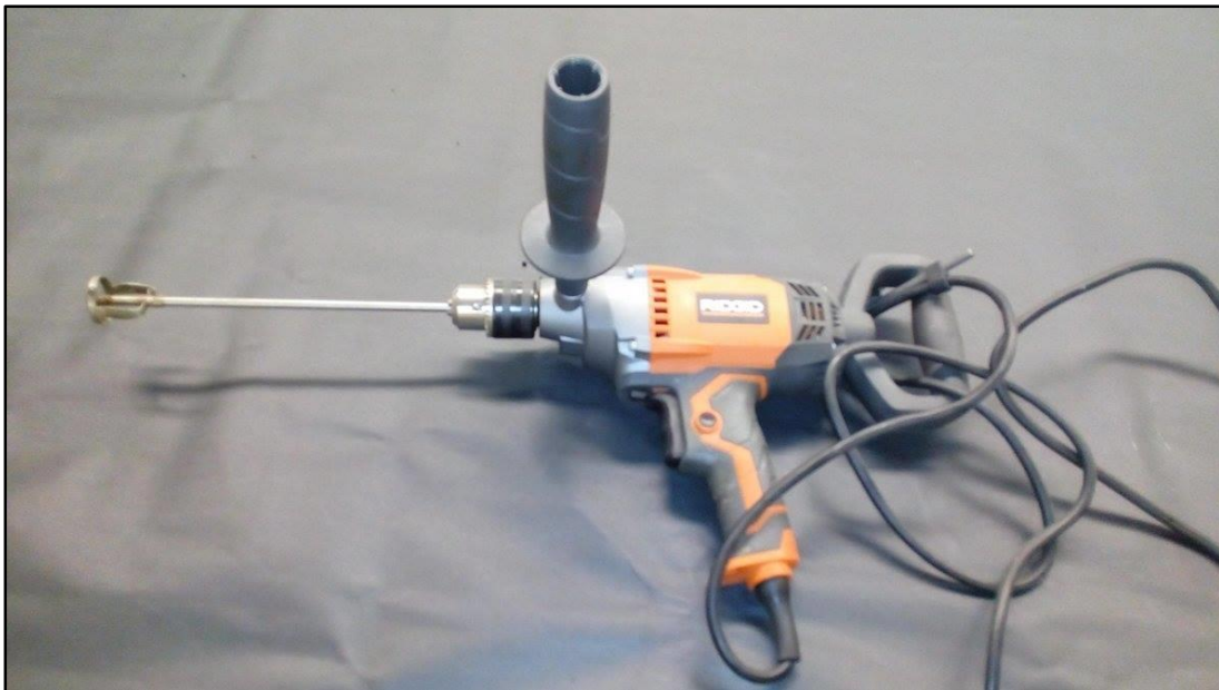
Figure 3.11 Jiffy mixer used for epoxy mixing
