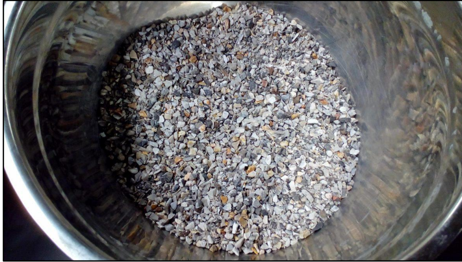
Figure 3.4 Pitcher, Oklahoma flint aggregate used in this study
