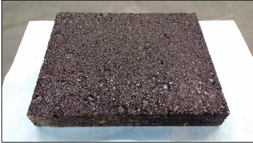
Figure 3.10 Compacted slab in kneading slab compactor
