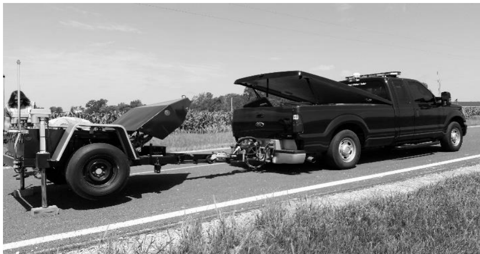
Figure 3.2 Locked Wheel Skid Trailer data collection
