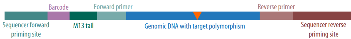
Figure 4-1. Primer and amplicon construction. The first round of PCR uses a forward primer containing the M13 sequence to amplify the target region. The second round of PCR extends from the M13 tail and incorporates a unique barcode, leading to a final product containing the sequencer primers, barcode, M13 sequence, and polymorphic target.
